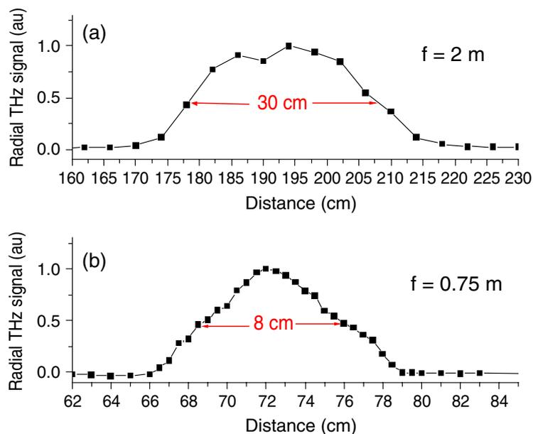
**Figure 4.** Radial THz signal as function of the propagation distance, measured along the filament for two different focal length lenses:  $f = 2$  m (a) and  $f = 0.75$  m (b). The full width at half maximum (FWHM) is the length of the obtained plasma channels.
