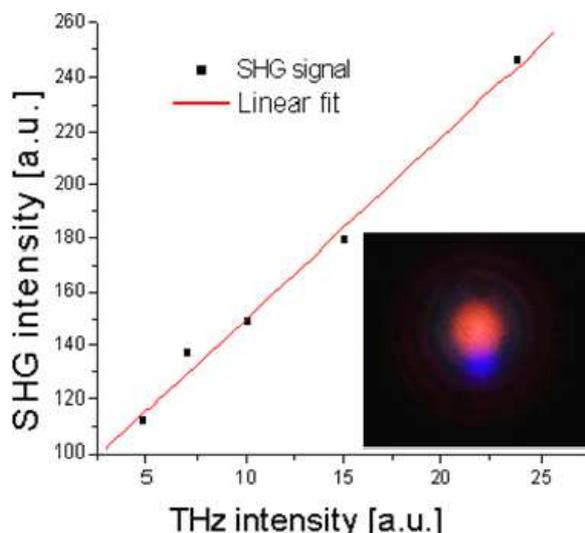
**Figure 9.** SHG signal versus the THz signal. The linear dependence of these two signals is an indication of SHG by the third-order mixing of the fundamental and THz pulses. The inset is a photographic picture of the conical emission coming from the filament. The blue spot that gives SHG signals is emitted off-axis and exhibits a 400 nm centered frequency spectrum.
