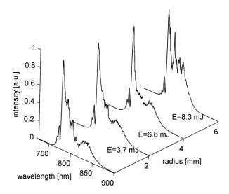
Fig. 3 Spectra measured behind 1 mm pinhole placed at different positions along the non-guided axis of the beam (the position  $\theta$  is the beam center). The pulse energies contained within the radii are also indicated.
