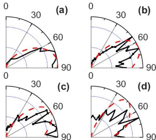
FIG. 5. Normalized radiation pattern measured at frequencies 655 MHz (a), 2.5 GHz (b), 1.55 GHz (c), 2.75 GHz (d) and for a plasma length  $L = 20$  cm (black curve). The dashed red lines show the corresponding radiation patterns calculated using formula (4).
