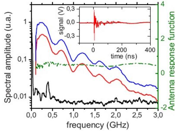
FIG. 3. Radiation spectrum (red curve) and background noise (black curve) measured with antenna A at 15 m and for  $\theta = 90^\circ$  with electrode A and an applied voltage of 40 kV. Antenna transfer function and deconvoluted spectrum are shown respectively as green dashed line and blue continuous line. The corresponding temporal waveforms for signal and noise are presented in the inset.
