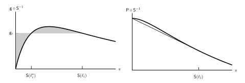
**Fig. 1** Graphical determination of the crack length  $l_i$  using the convexification of  $P \circ S^{-1}$ . The slope  $g_i := g(\ell_i)$  corresponds to the Maxwell line, i.e. the line giving the equality of the areas in the graph of  $g \circ S^{-1}$ .
