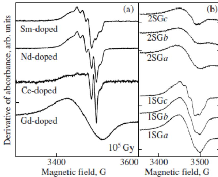
**Fig. 2.** Changes in the EPR spectra of various (a) *RE*-doped and (b) Sm- and Gd-codoped aluminoborosilicate glasses (defect region at  $g \sim 2$ ) plotted vs. Sm content for the following values of the Sm/Gd ratio: 1 : 3 (*SGa*), 1 : 1 (*SGb*), and 3 : 1 (*SGc*).
