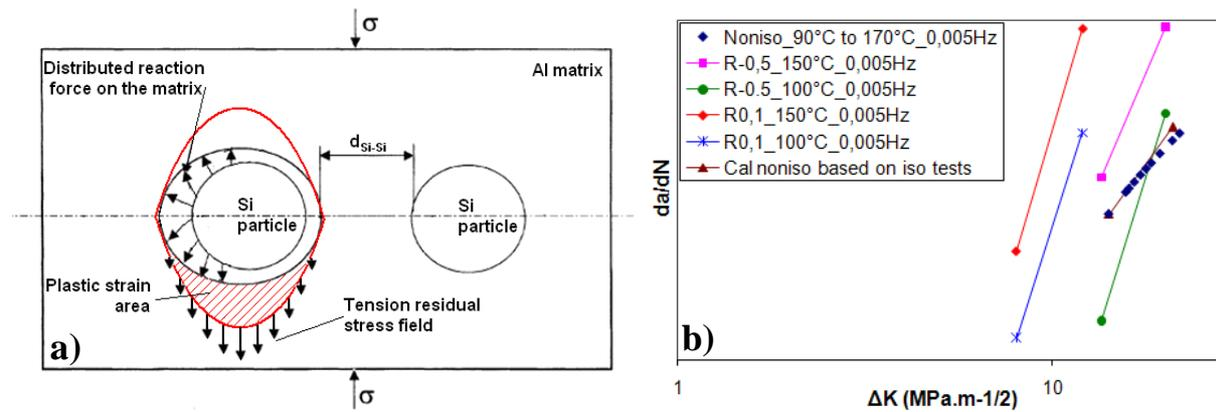
Figure 6 – a) A schematic showing the matrix/particle interface deformation, the engendered plastic strain area and the induced tension residual stress field, under remote compression load;
