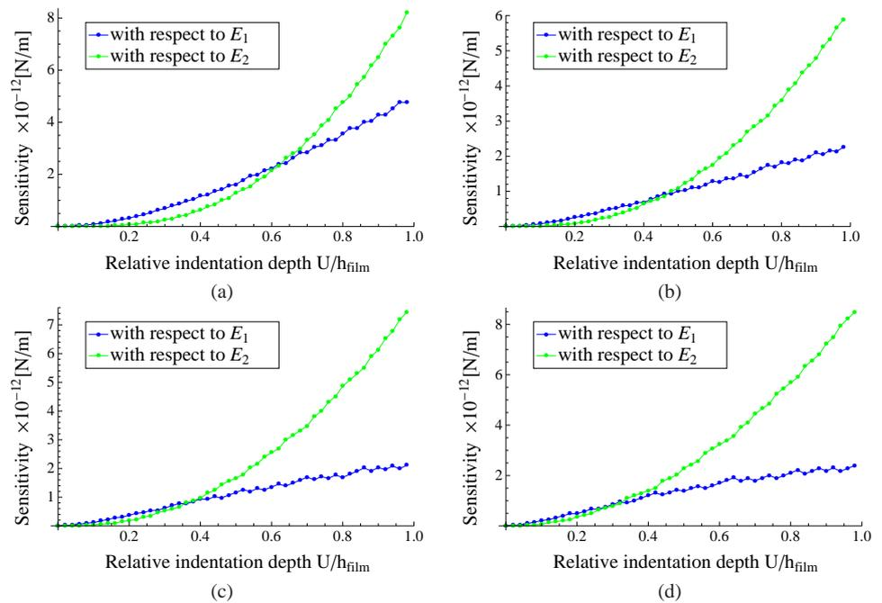
Fig. 7 Reaction force sensitivity with respect to  $E_1$  and  $E_2$  for: (a)  $E_1/E_2 = 0.5$ , (a)  $E_1/E_2 = 1$ , (c)  $E_1/E_2 = 2$ , (d)  $E_1/E_2 = 4$
