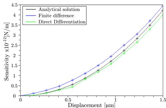
Fig. 6 Comparison of the sensitivities from finite difference and direct differentiation
