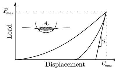
Fig. 1 Typical load displacement curve of the indenter
