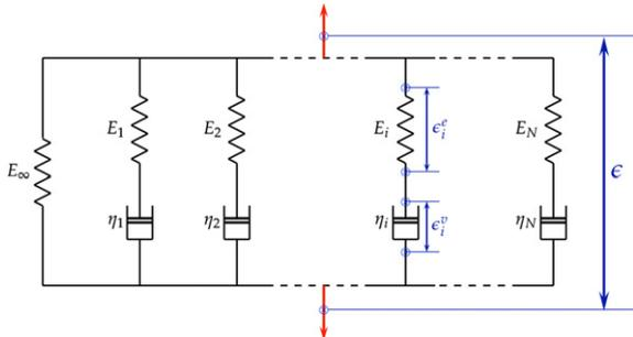
Fig. 6. Generalized Maxwell model with  $N$  viscoelastic elements.
