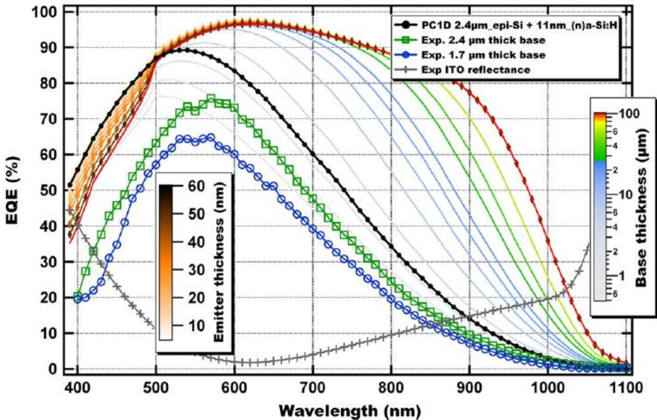
Figure 4. External quantum efficiencies obtained by PC1D simulations varying the emitter (5 to 60 nm) and the base (0.5 to 100  $\mu\text{m}$ ) thickness for the structure describe in Fig.1. Experimental EQE of our 1.7  $\mu\text{m}$  and 2.4  $\mu\text{m}$  cells is represented by the blue and green open symbols respectively.
