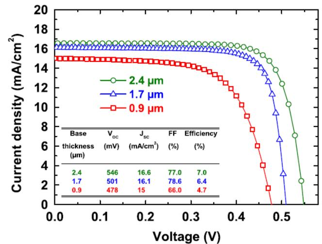
**Figure 2. Current-voltage characteristics of solar cells having three different thicknesses.**
