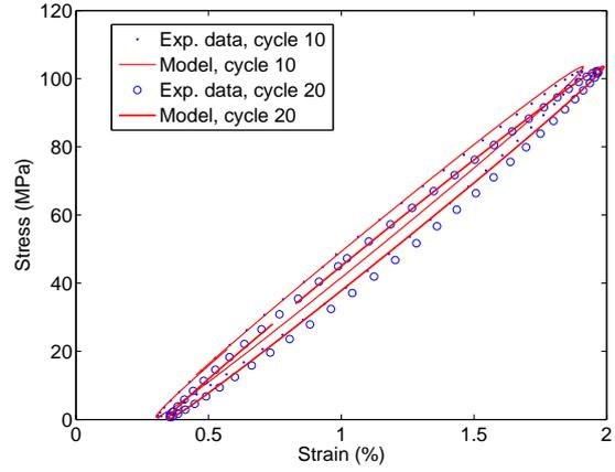
(b) Stress-strain response at cycles 10 and 20
