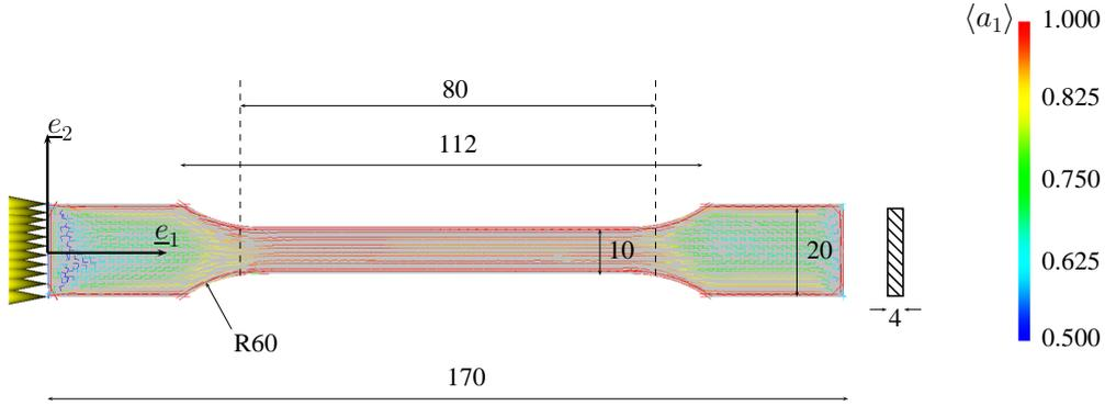
Figure 2: Injection simulation of the ISO527-2-1A tensile specimen with MOLDFLOW, and display of the average fibre orientation over the thickness  $\langle a_1 \rangle = \int_0^4 a_1(z) dz$ . 4242 triangular shell elements with 21 Gauss points through the thickness are used for the numerical computation (“Fusion analysis”).
