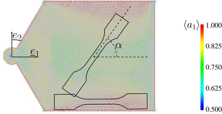
Figure 3: Injection simulation of the plate with MOLDFLOW, and display of the average fibre orientation over the thickness  $\langle a_1 \rangle = \int_0^2 a_1(z) dz$ . The plate dimension is  $100 \times 100 \times 2 \text{ mm}^3$  whereas the ISO527-2-5A tensile specimen length is 75 mm (gauge length 20 mm, section  $4 \times 2 \text{ mm}^2$ ). 5476 triangular shell elements with 21 Gauss points through the thickness are used for the numerical computation (“Fusion analysis”).
