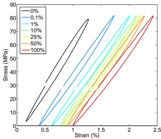
(a) Stress-strain response during fatigue test
