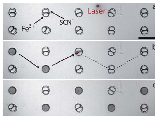
**Fig. 6** Laser induced merging of droplets in anchor sites. (a) Filled droplet array. Laser spot is shown as a red dot. (b) The laser is scanned in the pattern shown. As it stops on the droplet-droplet interface it initiates fusion and a chemical reaction takes place. The solid line shows where the beam has been, the dashed line its future path. (c) The laser completes its path leaving 5 anchor points with a reaction product and all other droplets undisturbed. Scale bar is 400  $\mu\text{m}$ .
