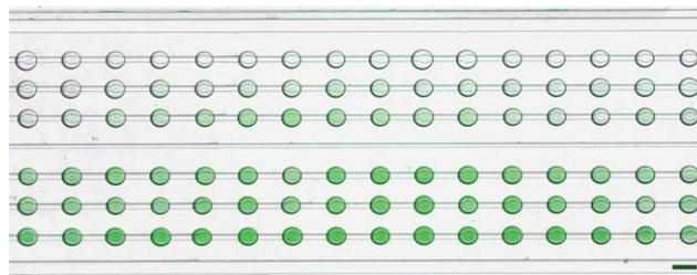
**Fig. 4** A superposition of bright-field and fluorescent images of a 96 anchor array. The droplet composition has been altered from pure water to a solution of water and green fluorescent beads to create a gradient. The droplet volume is 7 nL each. The scale bar is 300  $\mu\text{m}$ .
