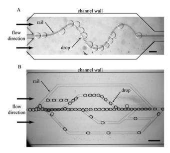
**Fig. 4** Microscope images of multiple water drops guided from left to right along microfabricated rails (50 μm in width and 50 μm in depth) in an external flow of fluorinated oil. (A) Large drops of radius  $R \approx 200$  μm follow a narrow sinusoidal rail inside a Hele-Shaw cell of height h = 100 μm. (B) Smaller drops of radius  $R \approx 50$  μm follow a complex network of rails with bifurcations and junctions inside a Hele-Shaw cell of height h = 50 μm. The scale bars represent 500 μm.
