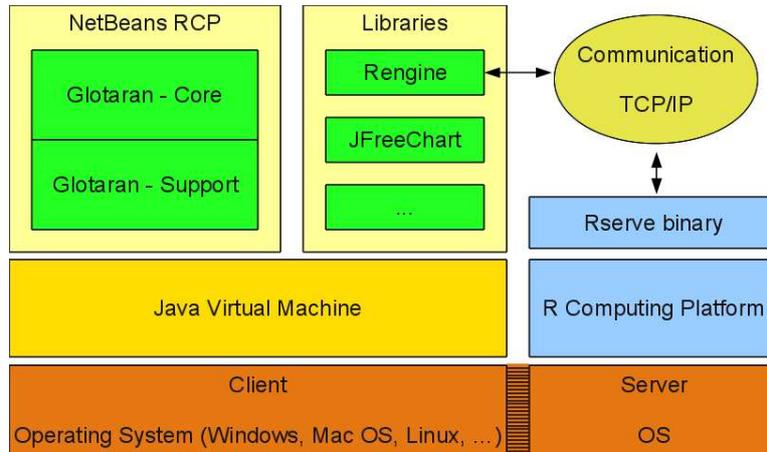
Figure 10: Application diagram showing the interaction between **Glotaran**, R and Java.
