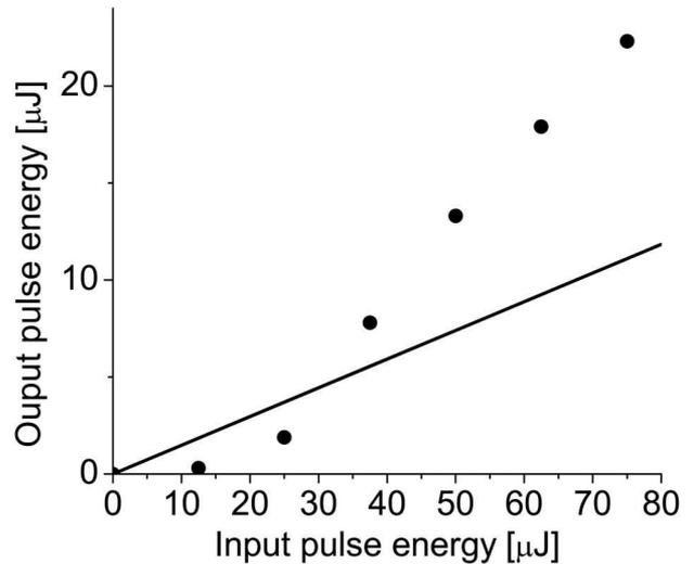
Fig. 5. Numerical simulation results of the PCD 10  $\mu\text{m}$  output pulse energy as a function of input 1.48  $\mu\text{m}$  pulse energy (dots), compared with the Manley–Rowe upper limit for single-stage DFM (solid line). Simulation parameters are explained in the text.
