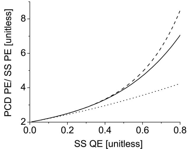
Fig. 3. Ratio of PCD to single-stage (SS) DFM power efficiency as a function of quantum efficiency for three different MIR wavelengths: 5  $\mu\text{m}$  (dotted curve), 10  $\mu\text{m}$  (solid curve), and 15  $\mu\text{m}$  (dashed curve).
