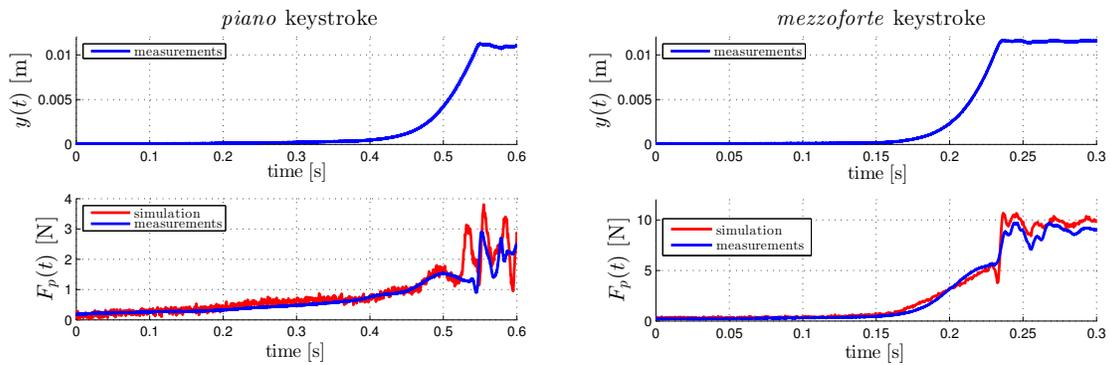
**Figure 2.** Top: measured position of the key  $y(t)$ , serving as an input for the simulation. Bottom: comparison between the simulated and the measured forces (see Fig. 1). Left: *piano* keystroke. Right: *mezzoforte* keystroke.
