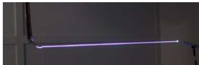
FIG. 4. Integrated image of guided Tesla discharges between two electrodes separated by 50 cm. The laser comes from the left and the applied voltage peak is 350 kV.
