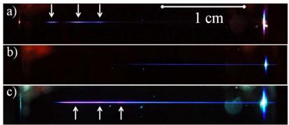
FIG. 1. Side view photography of the blue fluorescence of  $SiO_2$  induced by a self-guided laser pulse at a) 800 nm with  $P = 18 \, P_{cr}$ , b) 1.9  $\mu$ m with  $P = 13 \, P_{cr}$  and c) 1.9  $\mu$ m with  $P = 30 \, P_{cr}$ . The laser pulse is focused on a 70  $\mu$ m spot (FWHM) at the left surface of the 3 cm thick sample. Vertical arrows indicate the position of focusing-defocusing cycles.
