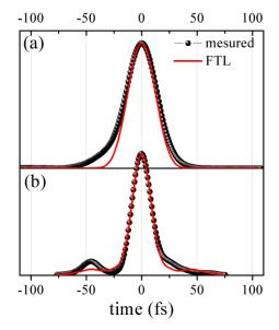
FIG. 3. Temporal pulse shape measured with the Wizzler for the initial pulse (40 fs FWHM) (a) and for filament lengths of 0.5 cm (20 fs FWHM) (b). Also shown in red is the Fourier Transform Limited pulse (FTL).
