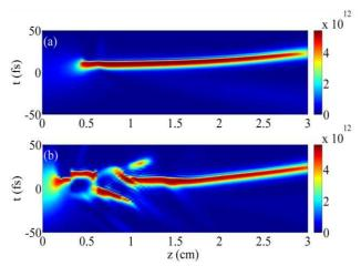
FIG. 5. Calculated time-space profile of the laser pulse for a laser pulse energy of 6  $\mu$ J (a) and 26  $\mu$ J (b) corresponding respectively to 7 and 30  $P_{cr}$ .
