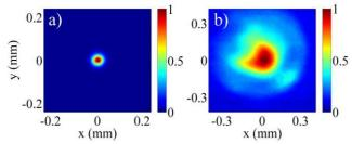
FIG. 2. Beam profile of the laser pulse at  $1.9 \, \mu m$  (a) with filamentation (b) without filamentation. Intensity scale is normalized.
