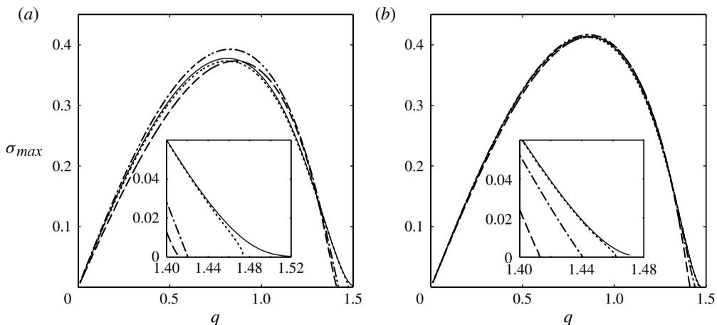
FIGURE 7. Maximum growth rate  $\sigma_{r \max}$  for (a)  $m = -4$  and (b)  $m = -8$  as a function of  $q$ . The exact growth rate is shown by a solid line and the different asymptotic approximations are shown by:  $-\cdot-$ , (3.25);  $---$ , Leibovich and Stewartson formula (4.4);  $\cdots$ , (6.2). The inset shows a close-up view of the range  $q = 1.4-1.5$ .
