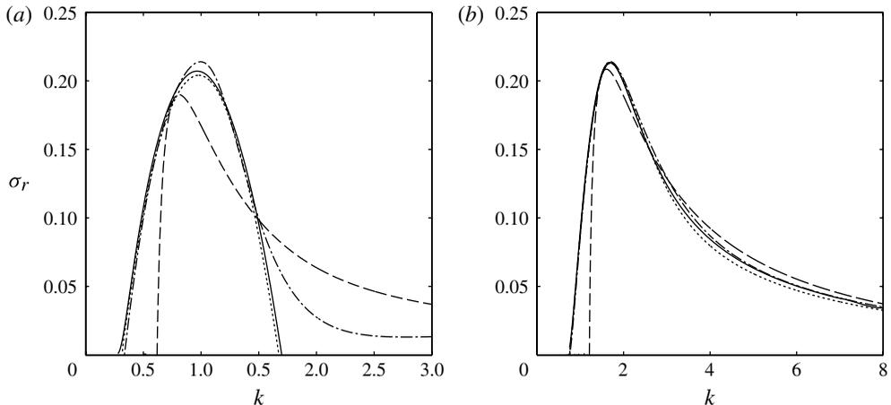
FIGURE 3. Growth rate  $\sigma_r$  for the azimuthal wavenumbers (a)  $m = -4$  and (b)  $m = -8$  as a function of the axial wavenumber  $k$  for the Batchelor vortex for  $q = 0.3$ . The exact growth rate is shown by a solid line and the different asymptotic approximations are shown:  $-\cdot-$ , (3.25);  $---$ , Leibovich & Stewartson formula (D 1);  $\cdot\cdot\cdot$ , (6.2).
