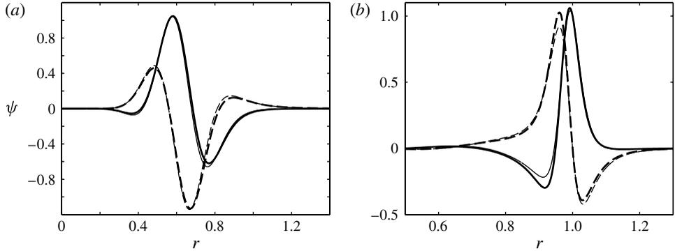
FIGURE 11. Comparison between the exact eigensolution (bold lines) and the WKB approximation (B 1) (thin lines) for (a) the Batchelor vortex for  $q = 0.8$ ,  $m = -8$ ,  $k = 3$  and (b) the Carton and McWilliams vortex for  $\alpha = 4$ ,  $\gamma = 2$ ,  $W_0 = 0.3$ ,  $m = -5$ ,  $k = 15$ . The solid and dashed lines show the real and imaginary part, respectively.
