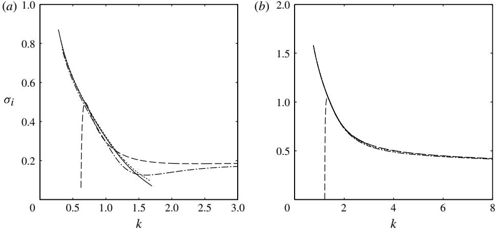
FIGURE 4. Frequency  $\sigma_i$  for the azimuthal wavenumbers (a)  $m = -4$  and (b)  $m = -8$  as a function of the axial wavenumber  $k$  for the Batchelor vortex for  $q = 0.3$ . The exact frequency is shown by a solid line and the different asymptotic approximations are shown:  $-\cdot-$ , (3.25);  $---$ , Leibovich and Stewartson formula (D 1);  $\cdots$ , (6.2).
