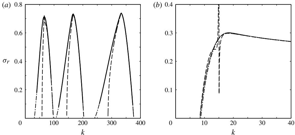
FIGURE 10. Growth rate  $\sigma_r$  for the basic flow (6.3) as a function of the axial wavenumber  $k$  for (a)  $m = -10, -25, -50$  (from left to right) and  $\alpha = 4, \gamma = 2, W_0 = 0.3$  and for (b)  $m = -6$  and  $\alpha = 2, \gamma = 4, W_0 = 0.2$ . The exact growth rate is shown by solid lines. The asymptotic growth rate (3.25) and (D1) are plotted with dash-dotted lines and dashed lines, respectively.
