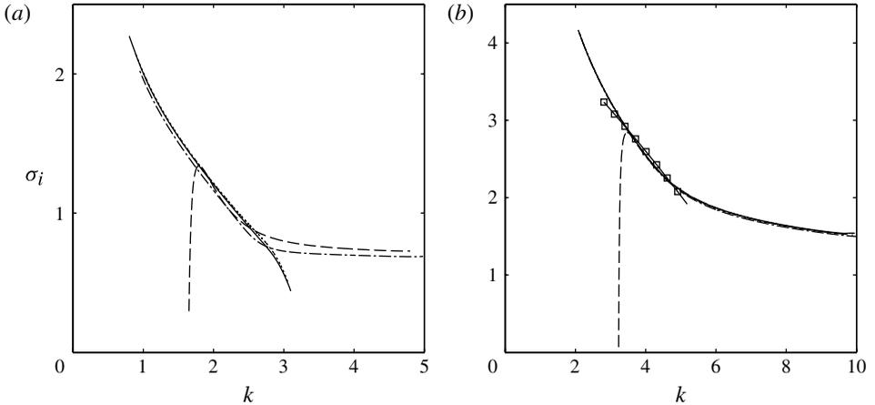
FIGURE 2. Frequency  $\sigma_i$  for the azimuthal wavenumbers (a)  $m = -4$  and (b)  $m = -8$  as a function of the axial wavenumber  $k$  for the Batchelor vortex for  $q = 0.8$ . The exact frequency is shown by a solid line and the different asymptotic approximations are shown:  $-\cdot-$ , (3.25);  $---$ , Leibovich and Stewartson formula (D 1);  $\cdots$ , (6.2). In (b), the asymptotic formula (4.20) of Di Pierro & Abid (2010) is also plotted with a solid line marked with square symbols.
