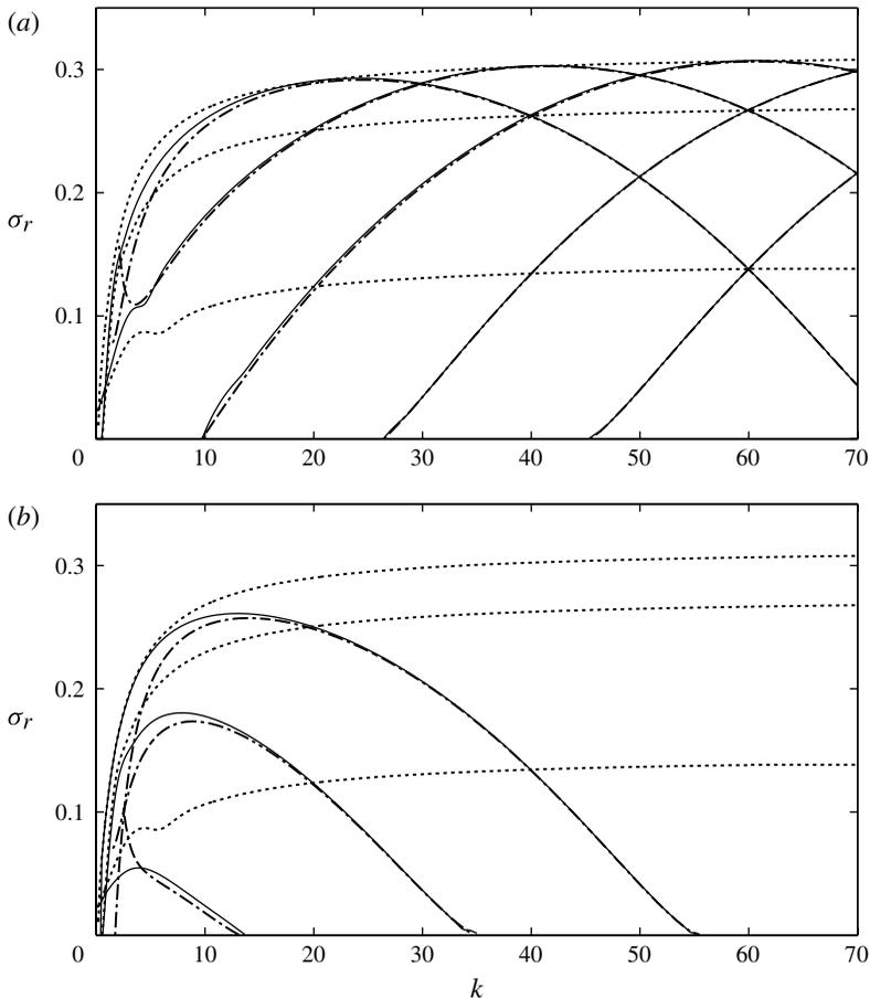
FIGURE 8. Growth rate  $\sigma_r$  for (a)  $m = -1, -2, -3, -4, -5$  (from left to right) and (b)  $m = 0, 1, 2$  (from top to bottom) as a function of the axial wavenumber  $k$  for the basic flow (6.3) with  $\alpha = 2$ ,  $\gamma = 2$  and for  $W_0 = 0$  (dotted lines) and  $W_0 = 0.05$  (solid lines). The asymptotic approximation (3.25) for  $W_0 = 0.05$  is plotted with dash-dotted lines.
