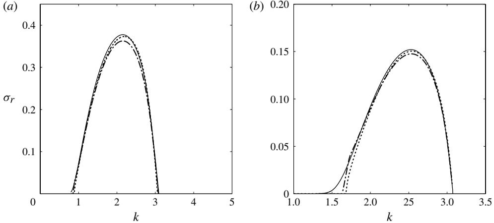
FIGURE 12. Growth rate  $\sigma_r$  for the azimuthal wavenumber  $m = -4$  for (a)  $q = 0.8$  and (b)  $q = 1.3$  as a function of the axial wavenumber  $k$  for the Batchelor vortex. The solid line shows the exact growth rate, the dotted line represents (6.2) and the dash-dotted line shows the approximation derived in appendix C.
