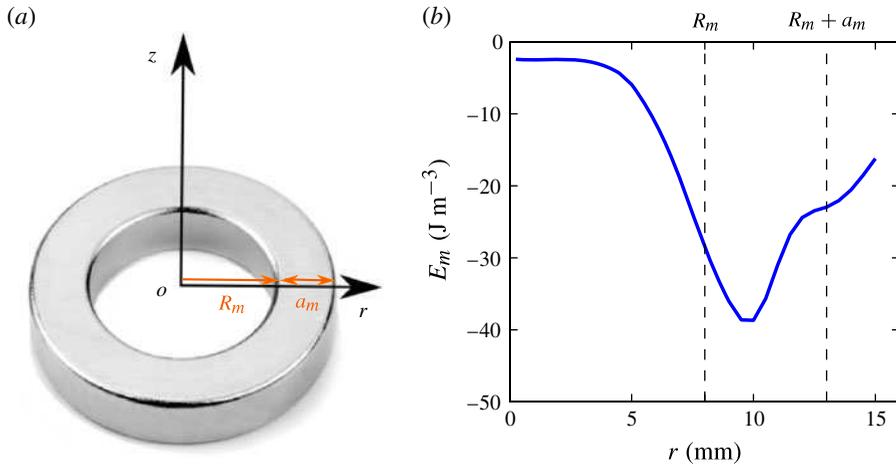
FIGURE 1. (a) Annular neodymium magnet of inner radius  $R_m = 8$  mm, width  $a_m = 5$  mm and height of 5 mm. (b) Magnetic energy per unit volume  $E_m$  as a function of radial coordinate  $r$  for this magnet, at a given distance  $z = 2$  mm above it. Dashed lines represent the position of the magnet.
