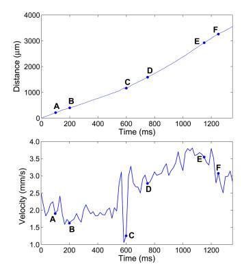
FIG. 4. Abscissa (top) and speed (bottom) of the rear interface along the channel as a function of time at bifurcation B, positioning events pointed out in Figure 2. The origin of distances is arbitrary.
