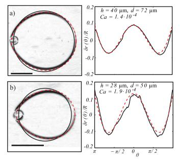
FIG. 3 (color online). Left: Images of anchored droplets deformed by the flow of oil. The dashed lines show the prediction from Eq. (7), while the solid line shows the equivalent circle of radius R. Scale bars represent 200  $\mu$ m. Right: Comparison between the deformations  $\delta r(\theta)/R$  extracted from the microscope images on the left (solid line) and the theoretical curve (dashed line) obtained from Eq. (7), using 9 as a prefactor.
