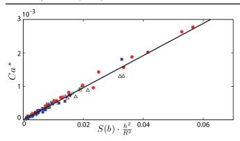
FIG. 4 (color online). Critical capillary number  $Ca^*$  plotted against  $S(b)h^2/R^2$  for the channel geometries, liquids, and surfactants as listed in the legend of Fig. 2. The solid line is a linear fit of the data.
