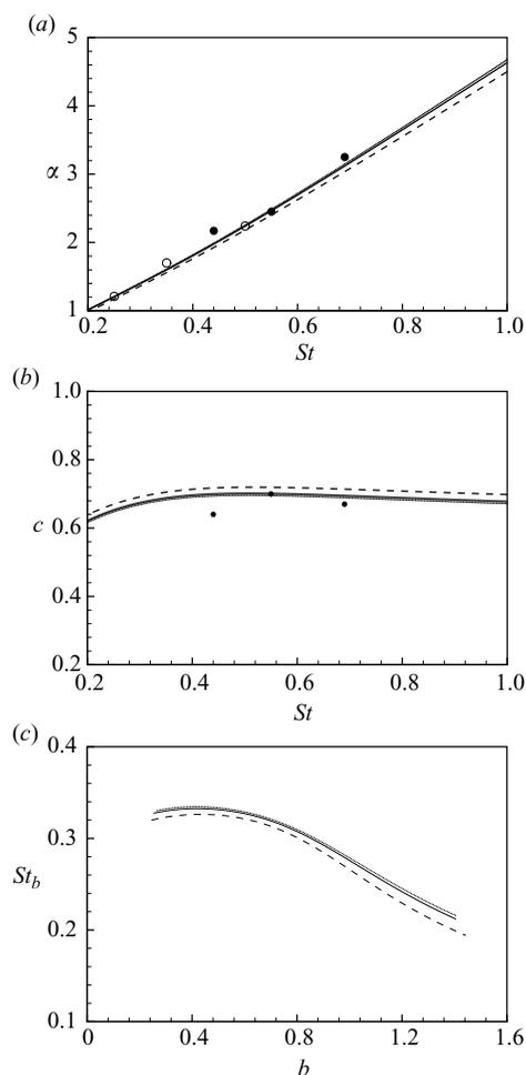
FIGURE 1. (a) Wavenumbers  $\alpha$ , (b) phase speed  $c$  of neutral modes versus frequency  $St$  and (c) Strouhal number  $St_b \equiv bSt$  versus  $b$ : dotted lines,  $M=0.3$ ; solid lines,  $M=0.5$ ; dashed lines,  $M=0.9$ ;  $\circ$ , experiment of Suzuki & Colonius (2006) ( $M=0.5$ );  $\bullet$ , experiment of Stromberg *et al.* (1980) ( $M=0.9$ ).
