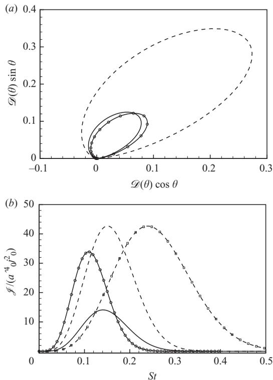
FIGURE 10. The (a) directivity and (b) spectrum of the acoustic field radiated by a linear wavepacket with  $St = 1.0$  at  $R = 1800$ . Solid lines:  $\sigma_s = 0.043$  and  $\Delta\omega = 0.5$ ; solid lines with symbols:  $\sigma_s = 0.0215$  and  $\Delta\omega = 0.5$ ; dashed lines without symbols:  $\sigma_s = 0.043$  and  $\Delta\omega = 0.8$ . In (b), the dashed line with symbols represents the spectrum at  $\theta = 55^\circ$  ( $\sigma_s = 0.043$  and  $\Delta\omega = 0.8$ ).
