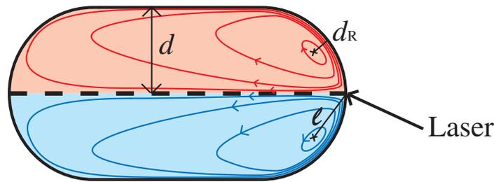
**Figure 2.** Sketch of the thermocapillary flow pattern inside a drop held by a laser centered in the test channel. The separatrix (dashed line) divides the drop into two regions, corresponding to two counter rotating rolls.
