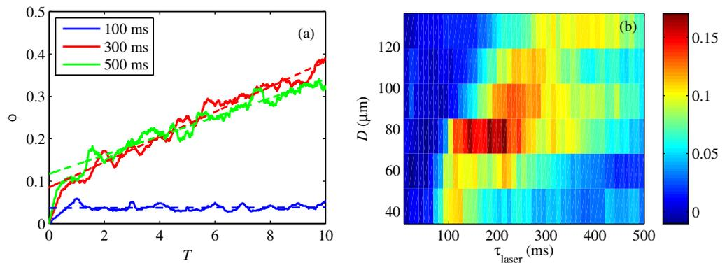
**Figure 10.** (a) Fraction of particles that cross the mid-plane of the drop as a function of time (solid line), and linear fit (dashed line), for  $D = 105 \mu\text{m}$  and different values of  $\tau_{\text{laser}}$ . (b) Mixing rate as a function of the distance between the laser spots  $D$  and the forcing time  $\tau_{\text{laser}}$ . The scale bar is in units of  $\text{s}^{-1}$ .
