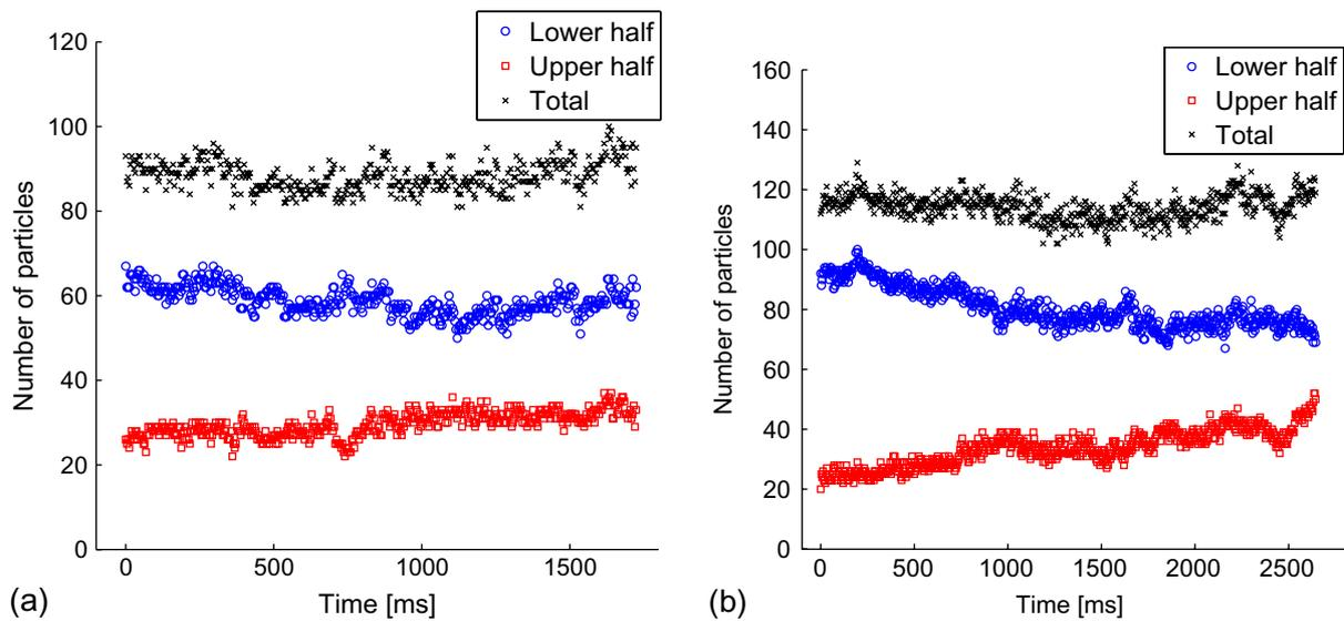
**Figure 7.** Number of tracers in the upper and lower halves of the drop as a function of time, while the drop is blocked by two alternating laser beams separated by a distance of  $17 \mu\text{m}$  (a) or  $89 \mu\text{m}$  (b). In both cases  $\tau_{\text{laser}} = 200 \text{ ms}$ .
