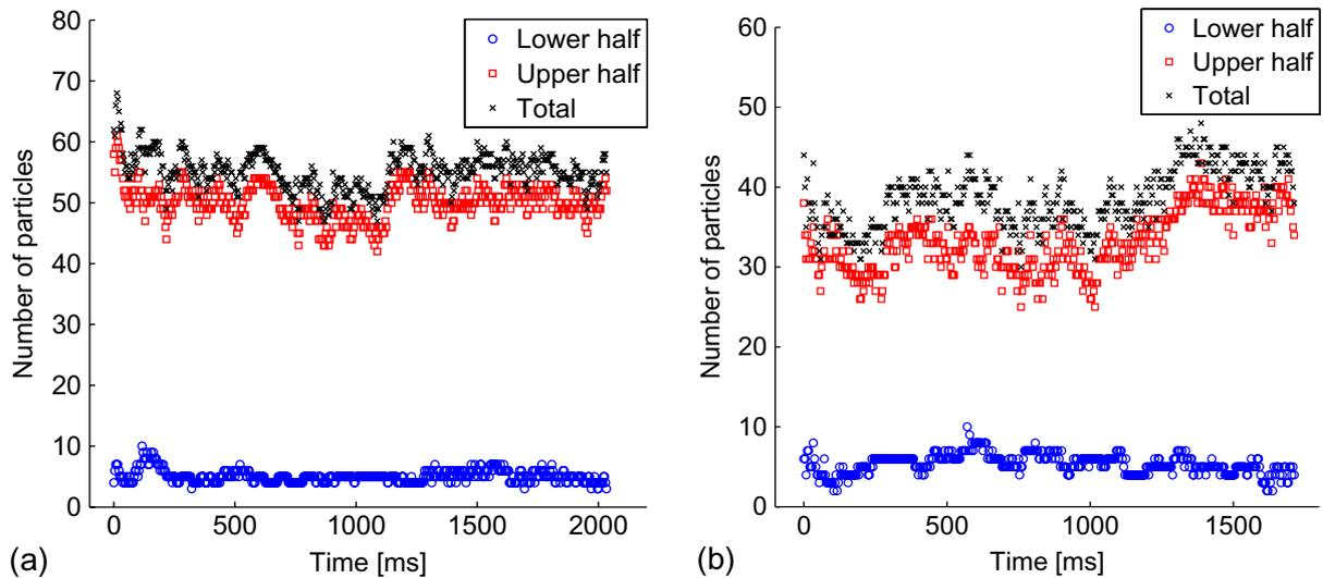
**Figure 6.** Number of tracers in the upper and lower halves of the drop as a function of time, while the drop is blocked by two stationary laser beams separated by a distance of  $16 \mu\text{m}$  (a) or  $86 \mu\text{m}$  (b).
