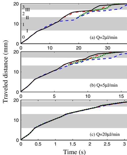
FIG. 2 (color online). Traveled distance along four paths as a function of time in the  $\mathcal{N}$  network. Driving flow rates: (a) 2, (b) 5, and (c) 20  $\mu\text{l}/\text{min}$ . The shaded and nonshaded areas represent successive generations.
