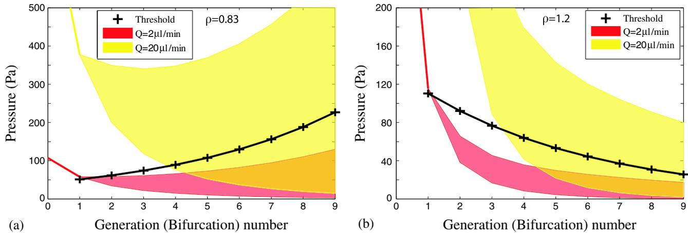
FIG. 5 (color online). Comparison of threshold pressures at every bifurcation to the pressures imposed in the straight channels by the driving flow rates  $Q = 2$  and  $20 \mu\text{l}/\text{min}$ . Labels on the  $x$  axis denote the bifurcation number for the threshold and the generation number for the viscocapillary pressure. (a)  $\mathcal{N}$  network and (b)  $\mathcal{W}$  network.
