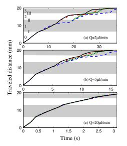
FIG. 2 (color online). Traveled distance along four paths as a function of time in the  $\mathcal{N}$  network. Driving flow rates: (a) 2, (b) 5, and (c) 20  $\mu$ l/min. The shaded and nonshaded areas represent successive generations.
