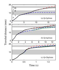
FIG. 3 (color online). Traveled distance in the W network. Driving flow rates: (a) 2, (b) 4, and (c) 20  $\mu$ l/min.
