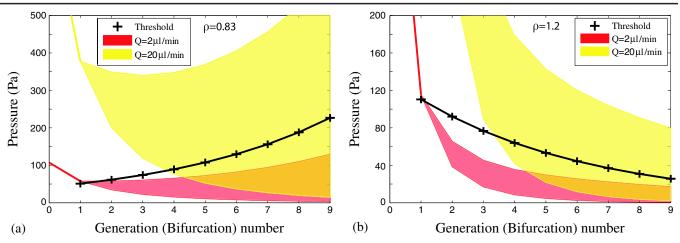
FIG. 5 (color online). Comparison of threshold pressures at every bifurcation to the pressures imposed in the straight channels by the driving flow rates Q = 2 and 20  $\mu$ l/min. Labels on the *x* axis denote the bifurcation number for the threshold and the generation number for the viscocapillary pressure. (a)  $\mathcal{N}$  network and (b)  $\mathcal{W}$  network.
