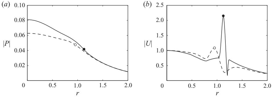
FIGURE 4. Eigenfunctions of the absolute mode in two homogeneous jets. —, marginally absolutely unstable profile (cf. figure 3a); - -, tanh-profile with  $b_u = 0.1$ . (a) Pressure  $|P(r)|$ ; (b) streamwise velocity  $|U(r)|$ . Circles mark the respective locations of the maximum baseflow velocity gradient. All eigenfunctions are normalized with respect to the value of  $|U|$  at  $r = 0$ .
