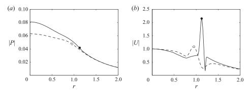
FIGURE 4. Eigenfunctions of the absolute mode in two homogeneous jets. —, marginally absolutely unstable profile (cf. figure 3a); - -, tanh-profile with  $b_u = 0.1$ . (a) Pressure |P(r)|; (b) streamwise velocity |U(r)|. Circles mark the respective locations of the maximum baseflow velocity gradient. All eigenfunctions are normalized with respect to the value of |U| at r = 0.
