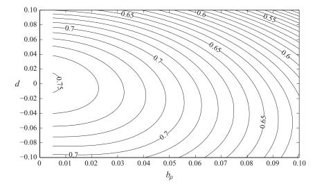
FIGURE 1. Critical density ratio  $S_{crit}$  for absolute/convective transition of hyperbolic-tangent profiles (3.1) and (3.2) with  $b_u = 0.05$ , as a function of  $b_\rho$  and d.
