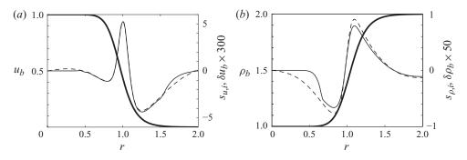
FIGURE 2. Baseflow profiles (3.1) and (3.2) with parameters  $b_u = b_\rho = 0.1$ , d = 0, S = 0.5, constrained optimal variations and sensitivities of the absolute growth rate. (a) —, velocity  $u_b$ ; —, variation  $\delta u_b$ ; – , sensitivity  $s_{u,i} = \text{Im}(s_u)$ ; (b) —, density  $\rho_b$ ; —, variation  $\delta \rho_b$ ; – , sensitivity  $s_{\rho,i} = \text{Im}(s_\rho)$ .
