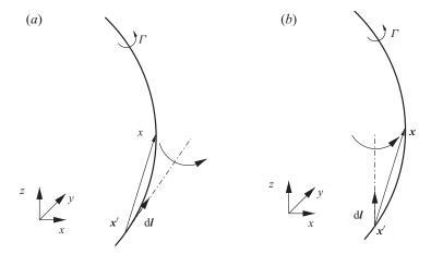
FIGURE 3. Graphical interpretation of the Biot-Savart law in homogeneous fluid (a) and quasi-geostrophic fluid (b). See explanations in text.
