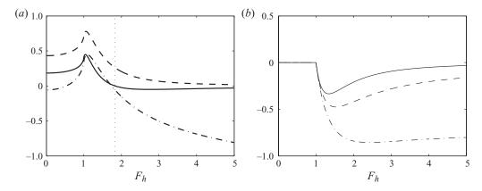
FIGURE 4. Real part (a) and imaginary part (b) of the parameters  $\mathscr{A}$  (---),  $\mathscr{B}$  (---) and  $\mathscr{D}$  (-·-) as a function of the Froude number  $F_h$  for the Lamb-Oseen vortex (4.7). The dotted line in (a) indicates the Froude number  $F_h = 1.83$  for which the real part of  $\mathscr{A}$  becomes negative.
