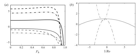
FIGURE 8. (a) Parameters  $\mathscr{E}_i$  as a function of the Froude number  $F_h$  for the Lamb-Oseen vortex (4.7).  $\mathscr{E}_1$  (——),  $\mathscr{E}_2$  (——) and  $\mathscr{E}_3$  (—·—) are shown by bold lines and  $\mathscr{E}_4$  (——),  $\mathscr{E}_5$  (——) and  $\mathscr{E}_6$  (—·—) by thin lines. (b) Coefficient  $\mathscr V$  describing viscous and diffusive effects as a function of 1/Ro for Sc=1 and  $F_h=0.1$  (——),  $F_h=0.5$  (——) and  $F_h=0.9$  (—·—).
