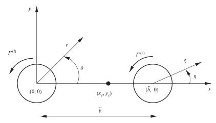
FIGURE 1. Sketch of the vortex pair in the frame of reference where it is steady. (x, y) are the Cartesian coordinates centred on the left vortex.  $(r, \theta)$  and  $(\xi, \eta)$  are the cylindrical coordinates centred on the left and the right vortex, respectively. The rotation centre of the vortex pair is located at  $(x_c, y_c)$ .
