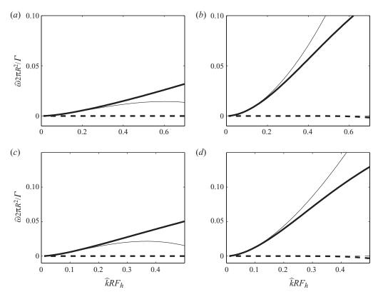
FIGURE 7. Comparison between the self-induction (thin solid line) for a Lamb-Oseen vortex in a strongly stratified ( $F_h = 0.5$ ) and rotating fluid and the exact frequency  $\omega_e$  of the slow bending mode m = +1 obtained numerically by a shooting method (real part: solid thick line; imaginary part: thick dashed line) for various Rossby numbers: (a) Ro = -2.5, (b) Ro = 2.5, (c) Ro = -1.25 and (d) Ro = 1.25.
