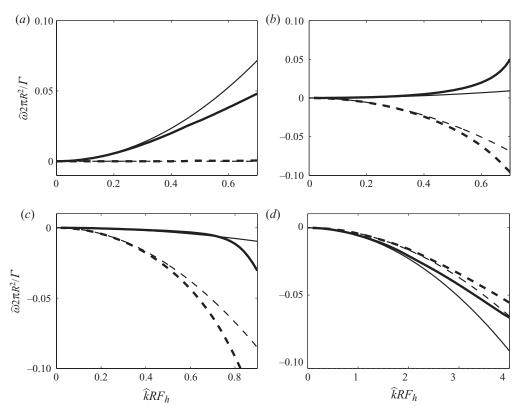
FIGURE 5. Comparison between the self-induction (real part: thin solid line; imaginary part: thin dashed line) for a Lamb-Oseen vortex in a stratified non-rotating fluid and the exact frequency  $\omega_e$  of the slow bending mode m=+1 obtained numerically by a shooting method (real part: thick solid line; imaginary part: thick dashed line) for various Froude numbers: (a)  $F_h = 0.9$ , (b)  $F_h = 1.67$ , (c)  $F_h = 2$  and (d)  $F_h = 10$ .
