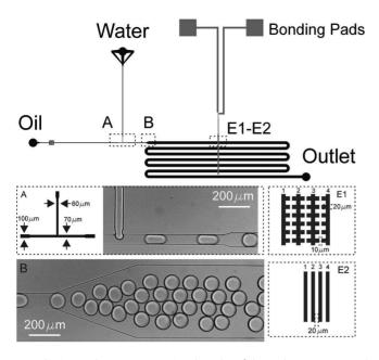
FIG. 1. Device geometry. A T junction (dimensions as reported in inset A) was used to form water emulsions in oil. Further downstream, channel width is 500  $\mu$ m (inset B) and microelectrodes were placed perpendicular to the flow direction (dimensions and patterns as reported in inset  $E_1$  and  $E_2$ ). Bonding pads were used to contact wires from excitation source. A square waveform was applied at the electrodes, with 1–3 and 2–4 sharing the same potentials.
