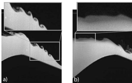
FIG. 1. Interfacial instabilities observed during experiments of two-layer exchange flow over a submerged sill with fluorescent dye diluted in the lower, saltier layer (Ref. 12). (a)  $\mathcal{KH}$  instability. (b)  $\mathcal{H}$  instability.
