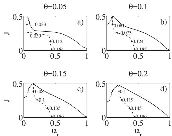
FIG. 8. Stability boundaries for  $R=1$  and  $a=0.05$  with the relative line of maximal amplification rates  $\omega_{i,\max}$ , for (a)  $\theta=0.05$ , (b)  $\theta=0.1$ , (c)  $\theta=0.15$ , and (d)  $\theta=0.2$ .
