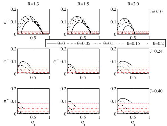
FIG. 13. (Color online) Amplification rates  $\omega_i$  vs the wavenumber for fixed values of the Richardson number  $J$  and for different values of the density scale parameter  $R$ . The larger amplification rates are those of  $\mathcal{KH}$  instabilities.
