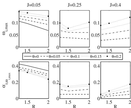
FIG. 12. Maximal amplification rates and corresponding wavenumber vs the density scale parameter  $R$  for fixed values of the Richardson number. The maximal amplification rates are found for the  $\mathcal{KH}$  modes.
