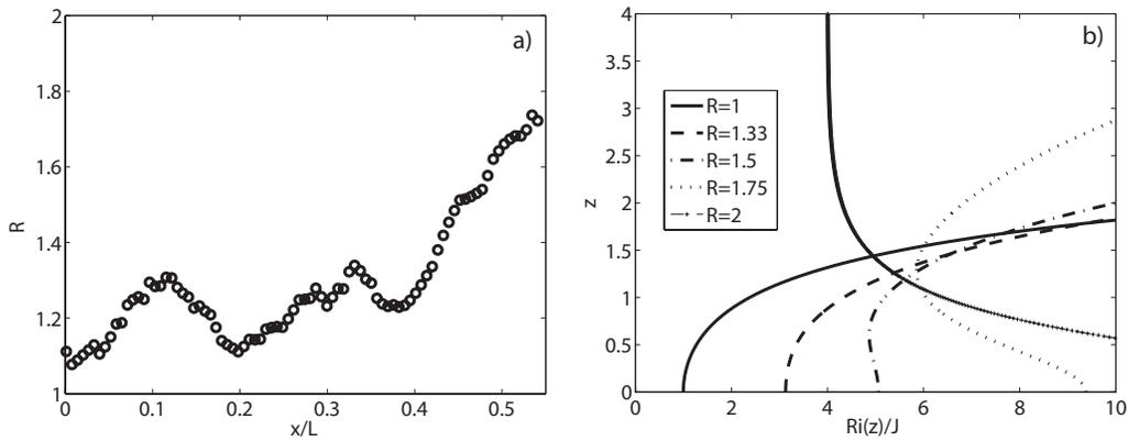
FIG. 9. (a) Experimental values for the density scale parameter  $R = \delta_r / \delta_\rho$  down a slope in the longitudinal direction, showing values ranging from 1 to 2. (b) Behavior of the ratio between the gradient and the local Richardson number  $Ri(z)/J = R \cosh^4(z) / \cosh^2(Rz)$  in the vertical direction  $z$  for different values of the parameter  $R$ .
