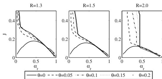
FIG. 10. Transitions boundaries from  $\mathcal{KH}$  to stable flow for different slope angles,  $R=1.33$ ,  $R=1.5$ , and  $R=2.0$  and  $a=0.05$  (inviscid solution). The instability regions are increased for larger slope angles. Transition to stable flow occur at lower Richardson numbers and wavenumbers as the density scale parameter  $R$  increases.
