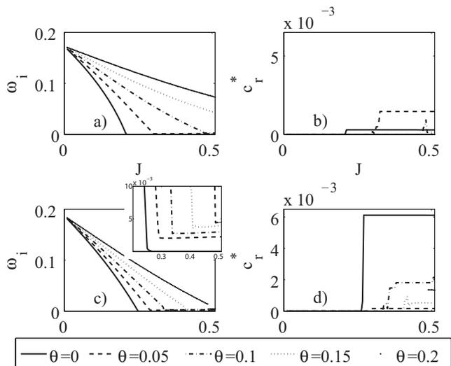
FIG. 4. Temporal amplification rates (left column) and intrinsic phase speed  $c_r^* = c_r - a$  (right column) with respect to the Richardson number  $J$  [(a) and (b)] for  $\alpha_r = 0.3$  and [(c) and (d)] for  $\alpha_r = 0.5$ ,  $R = 1$ , and  $a = 0.05$ . In (c) the area where the amplification rates drops to a nearly constant value are zoomed in the additional square.
