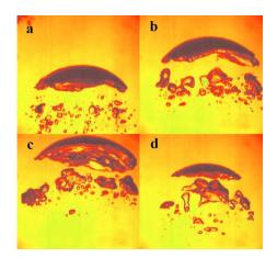
FIG. 3. (Color online) Pictures of typical crowned cap bubbles with, respectively, (a)  $V_{in}=114 \text{ cm}^3$ ,  $V_{sat}/V_{in}=0.05$ ; (b)  $V_{in}=126 \text{ cm}^3$ ,  $V_{sat}/V_{in}=0.15$ ; (c)  $V_{in}=144 \text{ cm}^3$ ,  $V_{sat}/V_{in}=0.3$ ; and (d)  $V_{in}=66 \text{ cm}^3$ ,  $V_{sat}/V_{in}=0.5$ .
