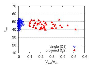
FIG. 7. (Color online) Measured opening angles  $\theta_m$  of single and crowned cap bubbles plotted vs the ratio  $V_{sat}/V_{in}$ . The data used to generate this figure are available online as supplemental material (Ref. 14).
