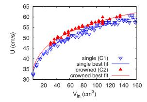
FIG. 4. (Color online) Rise speed U vs total injected volume of air for single cap bubbles ( $V_{sat}/V_{in} < 0.05$ ) generated with the C1 cup and crowned cap bubbles ( $V_{sat}/V_{in} > 0.1$ ) generated with the C2 cup. The best-fit curves have been computed by assuming  $U=\text{Fr }g^{1/2}V_{in}^{1/6}$  and then computing the best-fit Froude number Fr. The data used to generate this figure are available online as supplemental material (Ref. 14).
