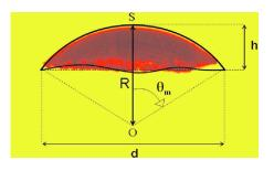
FIG. 2. (Color online) Geometry of a single spherical cap bubble. Picture of a single spherical cap bubble of air ( $V=68 \text{ cm}^3$ ) rising in still water at constant speed U. R is the radius of curvature of the bubble at the front stagnation point S, while  $\theta_m$  is its subtended half-angle; h and d are the height and width of the bubble, respectively.
