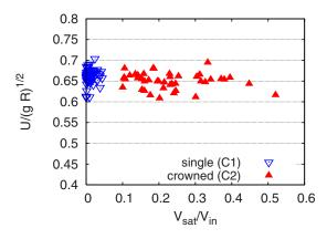
FIG. 6. (Color online) Measured individual Davies and Taylor ratios  $U/\sqrt{gR}$  of single and crowned cap bubbles plotted vs the ratio of the estimated volume  $V_{\text{sat}}$  contained in the satellite bubbles to the total injected volume of gas  $V_{\text{in}}$ . The ratio predicted by the theory of Davies and Taylor (Ref. 11) is  $2/3=0.666\overline{6}$ . The data used to generate this figure are available online as supplemental material (Ref. 14).
