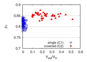
FIG. 5. (Color online) Measured individual Froude numbers of single and crowned cap bubbles plotted vs the ratio of the estimated volume  $V_{\text{sat}}$  contained in the satellite bubbles to the total injected volume of gas  $V_{\text{in}}$ . The data used to generate this figure are available online as supplemental material (Ref. 14).
