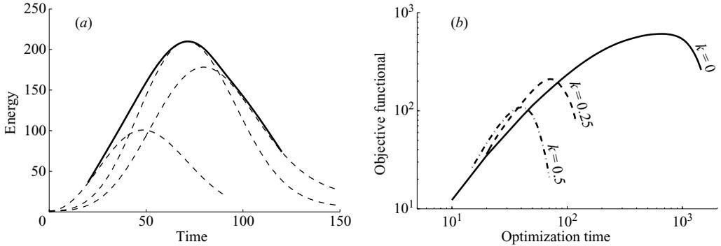
FIGURE 2. (a) Time evolution of the perturbation energy for  $k=0.25$  optimal disturbances at times  $T=20, 70, 120$  (dashed), at a Reynolds number  $Re=550$ . The envelope (solid) represents the maximum energy amplification that can be reached by  $k=0.25$  disturbances in the time interval  $20 < t < 120$ . (b) Maximum energy amplification in the time interval  $15 < t < 1500$  for perturbations at  $k=0$  (solid),  $k=0.25$  (dashed),  $k=0.5$  (dash-dotted) and  $Re=550$ .
