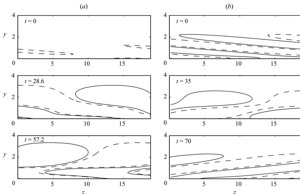
FIGURE 9. Chordwise vorticity contours in the  $(z, y)$ -plane of (a) an optimal Görtler–Hämmerlin perturbation and (b) a general optimal perturbation at  $k=0.25$  and  $Re=550$ . The successive snapshots were taken (from top to bottom) at times  $t=0$ ,  $t=T/2$  and  $t=T$ . For easier visualization the levels have been set at 2% and 20% of the maximum chordwise vorticity in (a) and (b) respectively.
