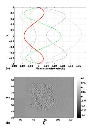
FIG. 5. (Color online) (a) The mean value of the total spanwise velocity in each upper box ( $z \ge 64$ ), shown in Fig. 4. Same color convention as in Fig. 4(b). (b) The spatial distribution of  $V_2$ . At the channel centerline, the total wall-normal velocity is equal to  $BV_2$ . Oblique waves are present at the wing tips of the spot (enhanced online).
