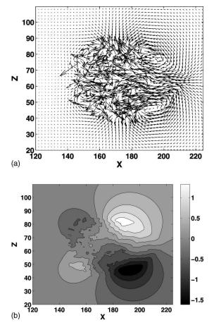
FIG. 9. (a) The flow field  $(U_0, W_0)$  exhibits a quadrupolar structure (not all the points are represented). (b) Spatial distribution of the stream function  $\Psi_0$ . Outside the spot, it has four lobes with alternating sign. Each lobe corresponds to a region of large recirculation.
