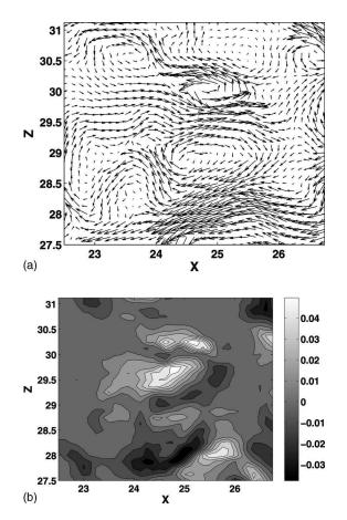
FIG. 12. (a) The flow field  $(U_0, W_0)$  depicted by vectors. Two dipoles are clearly observed. (b) The Reynolds stress  $U_0V_1$ . There are three *x*-elongated patches with positive value.
