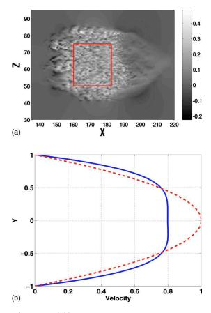
FIG. 3. (Color online) (a) Spatial distribution of  $U_1$ . In the turbulent region limited by the (red) box,  $U_1$  is mainly positive. (b) The mean profile of the total streamwise velocity (in solid blue). The laminar parabolic profile is shown with the dashed (red) line.
