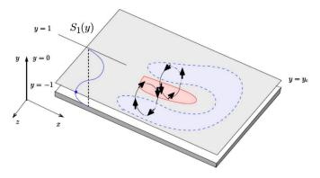
FIG. 11. (Color online) 3D reconstruction of the crescent vortex, depicted by  $V_1$  and  $(U_1, W_1)$  in Fig. 10. The distribution of  $V_1$  has a crescent shape in the shaded plane for some  $y=y_c \in [0, -1]$ . The two circles represent the cross section (z, y) of the streamwise vortices. The polynomial  $S_1$  is plotted by a solid blue line. For clarity, only the two counter-rotating streamwise vortices spanning the half-space  $y \in [-1, 0]$  are represented.
