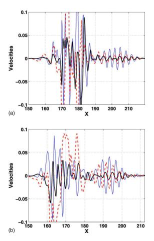
FIG. 7. (Color online) The profiles of  $U_2$  (in dashed red),  $W_2$  (in thin blue),  $V_2$  (in thick black) along a streamwise line for z=44 (a) and z=86 (b). The wave packets are clearly observed for  $x \in [190,215]$  (a) and  $x \in [180,210]$  (b).
