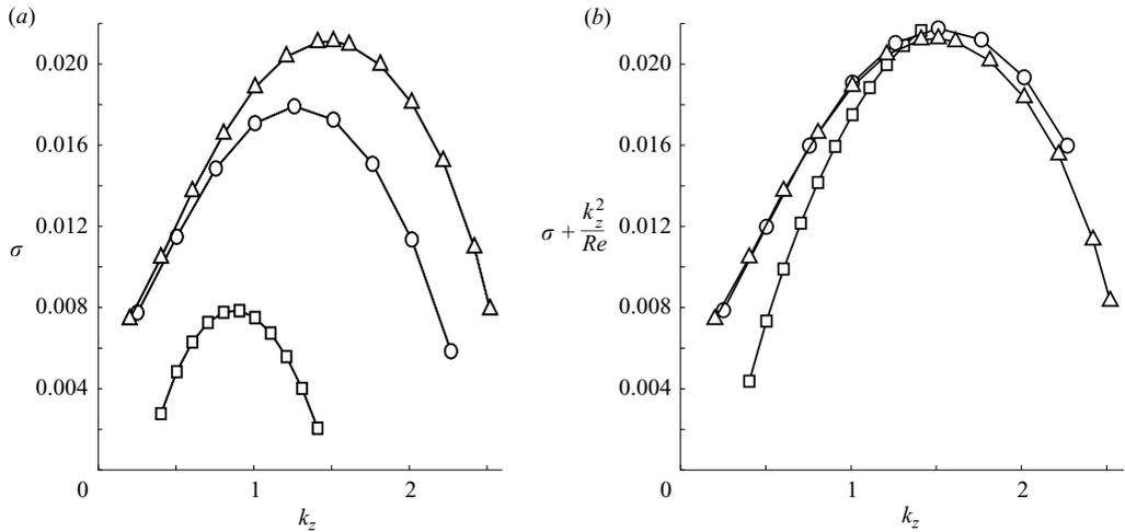
FIGURE 11. Plots of the growth rate of the zigzag instability for different Reynolds numbers: (a) growth rate as a function of  $k_z$ , (b) growth rate compensated for viscous damping against  $k_z$ .  $\square$ ,  $Re = 100$ ;  $\circ$ ,  $Re = 500$ ;  $\triangle$ ,  $Re = 16000$ . The Froude number is  $F_h = 1$ .
