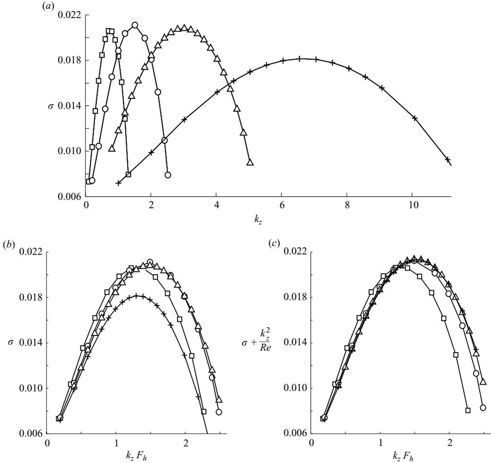
FIGURE 9. Plots of the growth rate of the zigzag instability for different low Froude numbers as a function of (a) the vertical wavenumber  $k_z$ , (b) the vertical wavenumber rescaled by the horizontal Froude number  $k_z F_h$ . In (c), the growth rate has been compensated for the viscous damping and plotted against  $k_z F_h$ .  $\square$ ,  $F_h = 1.7$ ;  $\circ$ ,  $F_h = 1$ ;  $\triangle$ ,  $F_h = 0.5$ ;  $+$ ,  $F_h = 0.2$ . The Reynolds number is  $Re = 16000$ .
