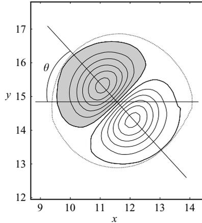
FIGURE 8. Vertical vorticity perturbation corresponding to an infinitesimal translation of one vortex of the basic state in the direction  $\theta$  that is to say  $\omega_z \propto (-\cos\theta(\partial/\partial x) + \sin\theta(\partial/\partial y))\omega_b$ . For other details see the legend of figure 7.
