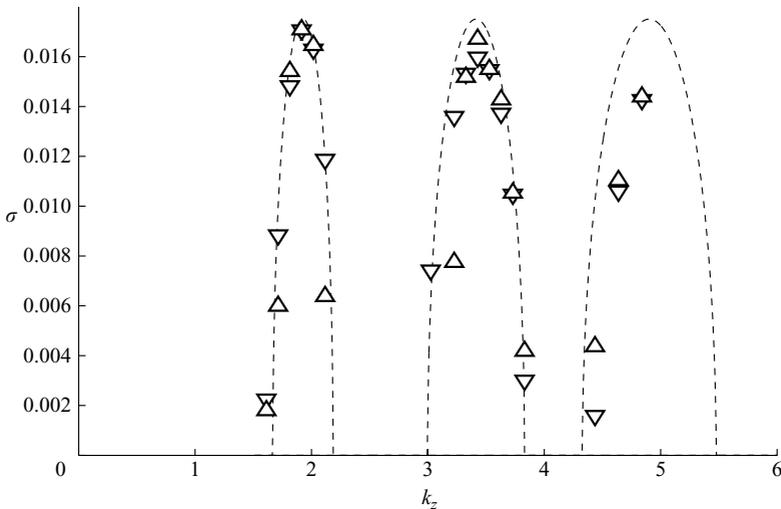
FIGURE 5. Plots of the growth rate of the elliptic instability as a function of the vertical wavenumber  $k_z$  for  $Re = 16\,000$ ,  $F_h = \infty$ , and  $\alpha_b = 0.15$ .  $\triangle$  and  $\nabla$  symbols show the growth rates of the symmetric and antisymmetric modes, respectively. The dash-dotted line represents the inviscid prediction of Le Dizès & Laporte (2002).
