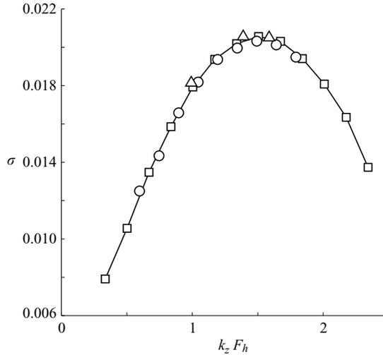
FIGURE 13. Plots of the growth rate as a function of the wavenumber times  $F_h$  for various initial distances between the vortices,  $\Delta$ ,  $b_0 = 6.75$ ,  $F_h = 1$ ;  $\square$ ,  $b_0 = 8$ ,  $F_h = 0.7$ ;  $\circ$ ,  $b_0 = 9$ ,  $F_h = 0.55$ . The other parameters are kept constant:  $M_x = M_y = 512$ ,  $L_x = L_y = 60$ ,  $\alpha_b = 0.15$ ,  $Re = 16000$ .
