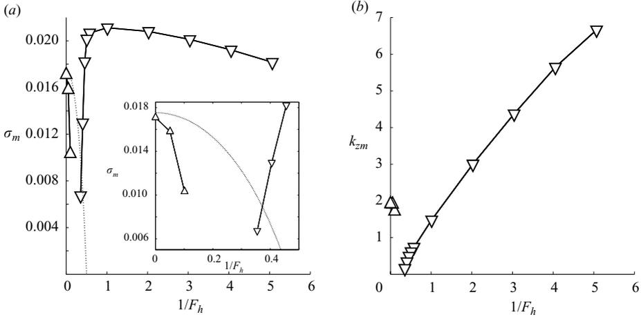
FIGURE 6. Evolution of (a) the maximum growth rate  $\sigma_m$  and (b) of the corresponding wavenumber  $k_{zm}$  as a function of the inverse of the horizontal Froude number for  $Re = 16000$  and  $\alpha_b = 0.15$ . The symbols  $\triangle$  and  $\nabla$  represent the elliptic and zigzag instabilities, respectively. The dotted line corresponds to the asymptotic value given by equation (4.3). A zoom on small  $1/F_h$  is included in the inset (a).
