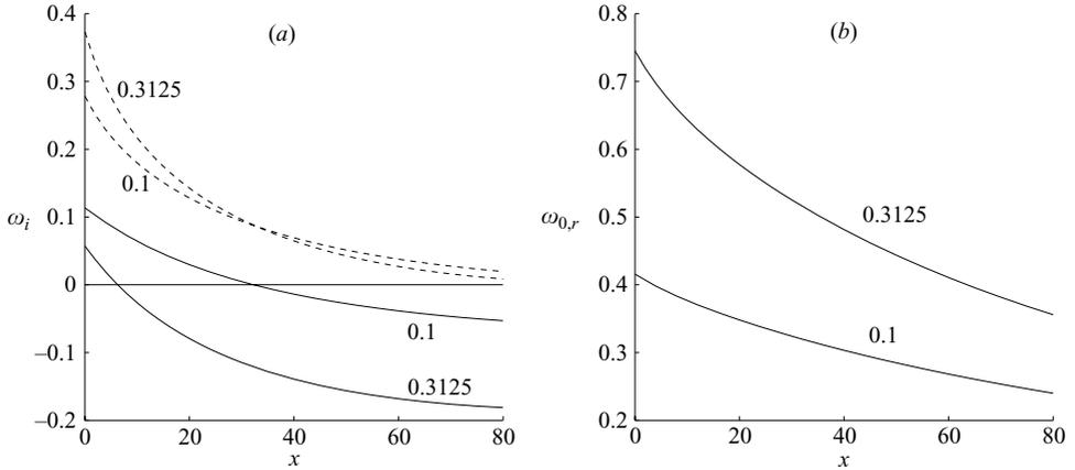
FIGURE 6. (a) Local absolute and maximum growth rates  $\omega_{0,i}$  (—),  $\omega_{i,max}$  (---) as functions of streamwise distance for  $S=0.3125$  and  $S=0.1$ . (b) Corresponding absolute frequencies  $\omega_{0,r}$ .
