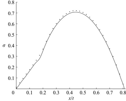
FIGURE 1. Comparison of the growth rate  $\sigma$  along spatio-temporal rays  $x/t$  as obtained from the numerical simulation (—) and from the dispersion relation ( $\cdot$ ) of a parallel jet with the parameters  $R/\theta = 20$ ,  $S = 0.57$ ,  $Re = 500$  and  $M = 0.1$ .
