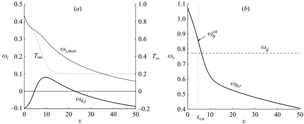
FIGURE 2. (a) Local absolute and maximum growth rates  $\omega_{0,i}$  (—),  $\omega_{i,max}$  (---) and ambient temperature  $T_\infty$  ( $\cdots$ ) as a function of streamwise distance  $x$ . (b) Comparison of the local absolute frequency  $\omega_{0,r}(x)$  (—) and the observed global frequency  $\omega_g$  (---).
