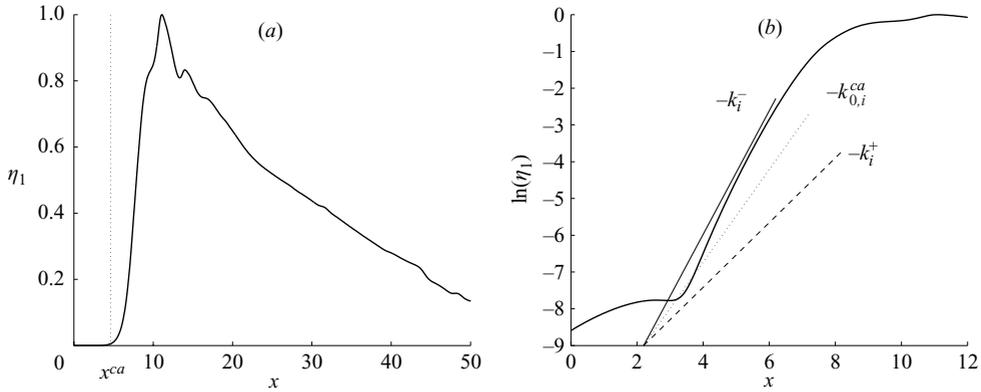
FIGURE 5. (a) Oscillation amplitude  $\eta_1$  as a function of streamwise distance. (b) Semi-logarithmic plot of the upstream front region; comparison of the front slope with spatial growth rates  $-k_{0,i}^{ca} = 1.26$ ,  $-k_i^+(\omega_0^{ca}, x=4) = 0.88$  and  $-k_i^-(\omega_0^{ca}, x=4) = 1.68$ .
