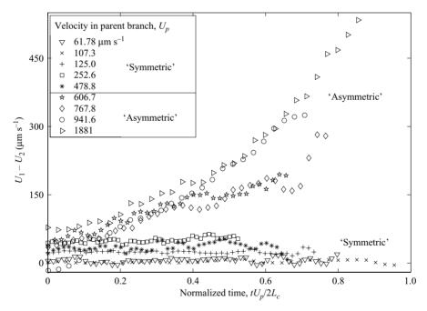
FIGURE 4. Evolution of the velocity difference for the fingers in the two daughter branches. At low flow rates, the velocity differences remain constant. When the velocity in the parent branch exceeds a threshold, the difference in the velocities increases rapidly. We refer to the two regimes as 'symmetric' and 'asymmetric', respectively.
