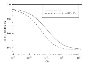
FIGURE 5. The fraction  $\alpha$  of the tube's cross-section that is occupied by the propagating finger as a function of the capillary number  $Ca = \mu \mathcal{U}/\sigma$  for tubes with square cross-sections. Results for tubes of rectangular, circular and elliptical cross-sections are qualitatively similar.
