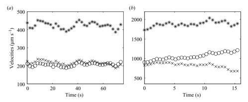
FIGURE 3. Time series of the velocity of the advancing fingers in channels  $1 (\circ)$  and  $2 (\times)$  as a function of time, for two different forcing flow rates. The sum of the two velocities (\*) remains approximately constant.
