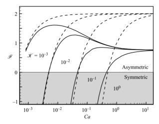
FIGURE 6. The function  $\mathscr{F}(Ca)$  for tubes of square cross-section, plotted for various values of the stiffness parameter  $\mathscr{K}$ . If  $\mathscr{F} < 0$  (> 0), the finger branches symmetrically (asymmetrically). The dashed lines represent the approximation  $\mathscr{F} = 2 - \mathscr{K}/Ca$  which provides excellent predictions for  $\mathscr{F}(Ca) = 0$ . Results for tubes of rectangular, circular and elliptical cross-sections are qualitatively similar.
