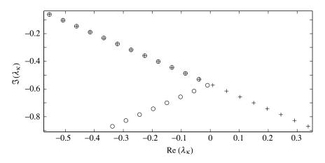
Figure 4. Locus of the first 20 eigenvalues of the CGL operator with supercriticality  $\delta = 3$  before (pluses) and after (circles) optimal control is applied (with  $\ell = 10^4$  and  $x_f = 47$ ). Note that, in this minimal-energy optimal control setting, the stable eigenmodes of the system matrix are unchanged, and the unstable eigenvalues of the system matrix are reflected across the imaginary axis.
