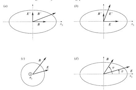
FIGURE 2. Cases 1, 2, 3 and 4 for a migration aligned with  $E \wedge B$ . (a) Possible settings  $B \| e_3$  or (E', B') in Case 1. (b) Possible settings  $E \| e_3$  or (E', B') in Case 2. (c) Case 3. (d) Case 4 with  $\theta = (E, e_3)$  and  $\varphi = (B, e_3)$ .
