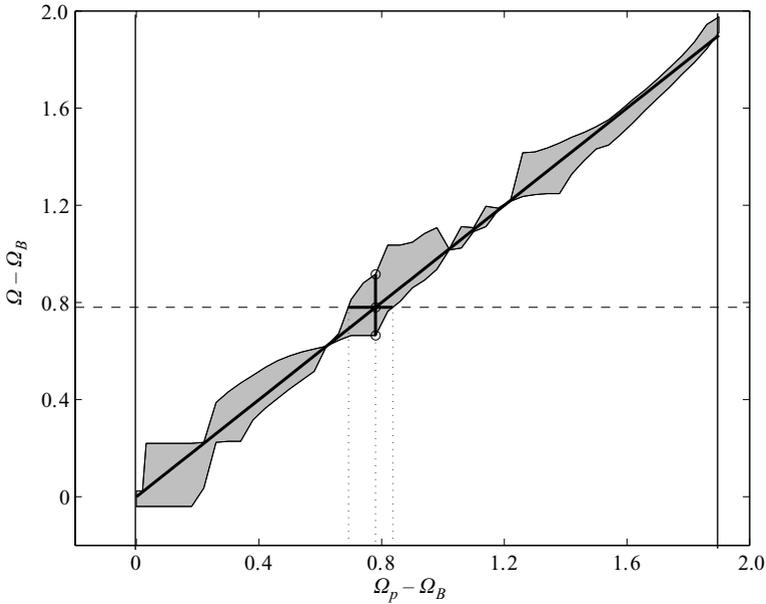
FIGURE 13. Robustness of control scheme with respect to uncertainties in parameter setting  $\Omega$ . Effective control range, defined in terms of the  $\Omega - \Omega_B$  interval as a function of nominal design swirl number  $\Omega_p - \Omega_B$  for  $N = 12$ ,  $\ell = 1$ .
