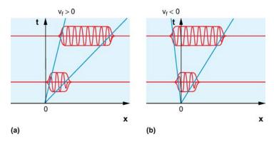
**Figure 7** Diagrams in the (x, t) plane, illustrating the dynamics of a saturated wave packet in an unstable flow, (*a*) nonlinear convective instability, the velocity  $v_f$  of the trailing front separating the saturated wave from the basic state is positive, (*b*) nonlinear absolute instability, the front velocity  $v_f$  is negative.
