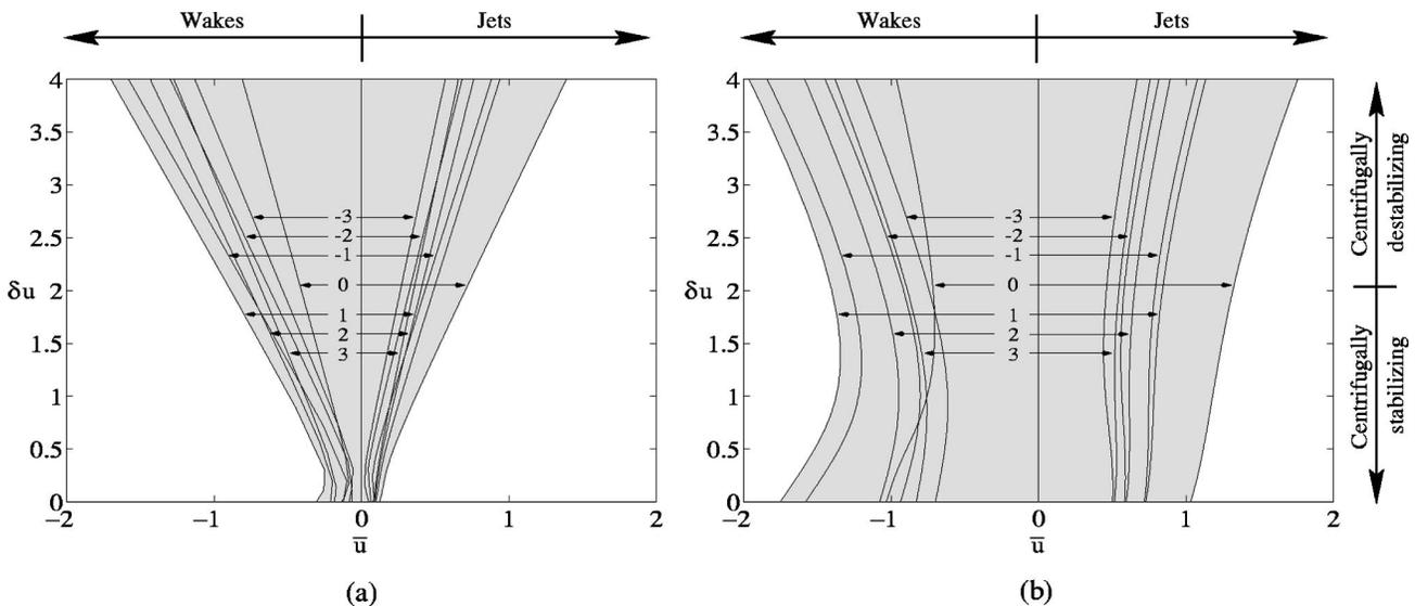
FIG. 5. AI/CI domains in the  $\bar{u} - \delta u$  plane for (a)  $\delta\gamma=1.5$  and (b)  $\delta\gamma=0.01$ . The shaded area corresponds to the absolute unstable region, and the clear area to the convectively unstable region.
