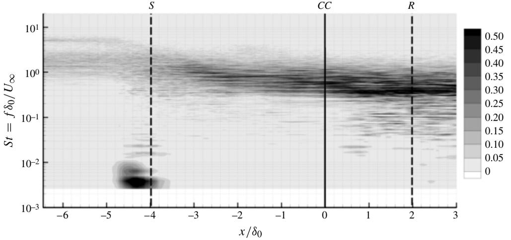
FIGURE 6. Contours of the weighted power spectral density of wall pressure in the  $St-x/\delta_0$ -plane. The power spectral density is normalized such that their integral over frequency is unity. Thirty contours levels have been used; the dashed vertical lines indicate the location of the separation  $S$  and reattachment point  $R$  respectively. The solid line indicates the position of the corner  $CC$ .
