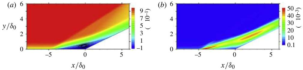
FIGURE 3. (a) Contours of the mean streamwise velocity field in the region of interaction, with 23 contour levels ranging from  $-0.1$  to  $1.0$ . Streamlines are indicating the recirculating flow region. (b) Streamwise-velocity fluctuation field  $\langle u'u' \rangle / U_\infty^2$  in the region of interaction, with 23 contour levels ranging from 0 to 0.058.
