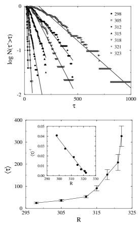
**Figure 5.** Top: distributions of transient lifetimes for a series of Reynolds numbers (quench experiments). Bottom: Characteristic times extracted from these distributions as functions of Re. Courtesy: S Bottin.
