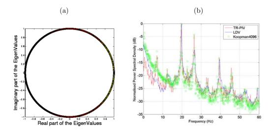
**Figure 3.** DMD of velocity fields in the longitudinal plane: (a) operator eigenvalues  $\lambda_k$ , well distributed on the unit circle. (b) Comparison between PSD obtained by Fourier transform of the LDV signal (solid blue line), amplitude spectrum of the DMD (green circles) and the mean value over space of the Fourier transform of the PIV snapshots (solid red line).
