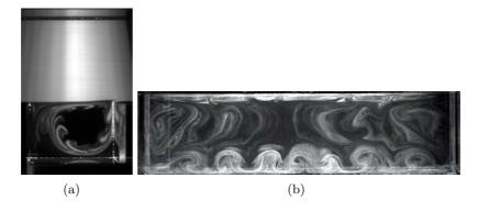
**Figure 2.** Smoke visualization for a cavity geometry L/H = 1.5, S/H = 6 and for a typical Reynolds number  $\Re_H \approx 3000$ . (a) Front view of the longitudinal plane (x, y), (b) top view of the spanwise plane (x, z) located at y/H = -0.3 inside the cavity.
