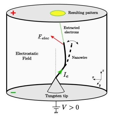
Fig. 1. Experimental settings: nanowire in field emission.
