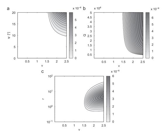
**Fig. 8.** Stability maps of the bi-articulated nanowire in field emission. (a) Influence of an initial tilting ( $Q = 20\,000$ , r = 4.458). (b) Influence of the quality factor (r = 4.458,  $\psi = 20^{\circ}$ ). (c) Influence of the time constant ratio ( $\psi = 20^{\circ}, Q = 20\,000$ ).
