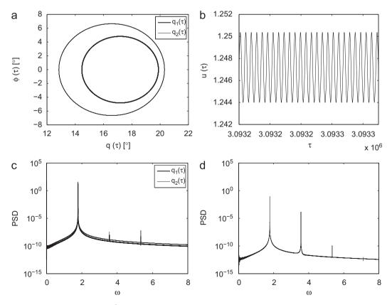
**Fig. 9.** Steady-state dynamic response for  $\nu = 1.55$  and  $\vec{Y}(0) = [q_1^0 q_2^0 U_0 0.01 0]$ . (a) Evolution of  $q(\tau)$  in the phase space. (b) Evolution of  $u(\tau)$ . (c) Frequency spectrum of  $q(\tau)$ . (d) Frequency spectrum of  $u(\tau)$ .
