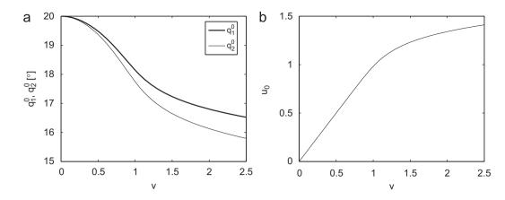
**Fig. 6.** Evolution of the fixed points  $(q_1^0, q_2^0, u_0)$  against v for  $\psi = 20^\circ$ . (a) Mechanical static equilibrium. (b) Electrical static equilibrium.
