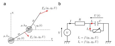
Fig. 3. Sketches of the NanoElectroMechanical System. (a) Mechanical contribution. (b) Electric contribution.
