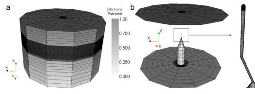
**Fig. 4.** 3D Finite element model of the electrostatic boundaries. (a) Outside view of the electrostatic box. (b) Nanowire:  $q_1 = 10^\circ$  and  $q_2 = -4^\circ$ .
