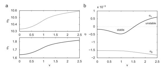
Fig. 7. Linear vibratory behaviour of the static equilibrium against v. (a) Evolution of the natural frequencies. (b) Evolution of the decay rates.
