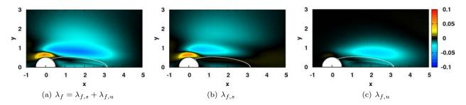
Figure 6. Growth rate of the neutral mode as a function of the location of the force  $(x_f, y_f)$ . The growth rate (a)  $\lambda_f$  is the sum of the two contributions, (b)  $\lambda_{f,s}$  and (c)  $\lambda_{f,u}$ , induced by, respectively, the steady and unsteady components of the force. The same colorbar is used in the three figures. Parameter:  $Re = Re_c = 46.8$ .
