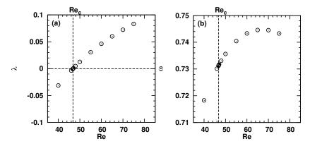
Figure 2. Global stability of the cylinder flow (without control). (a) Growth rate  $\lambda$  and (b) pulsation  $\omega$  (bottom) of the leading global mode as a function of the Reynolds number Re. The vertical dashed line outlines the threshold of the flow instability at  $Re_c = 46.8$ . The pulsation at the criticity is  $\omega_c \sim 0.73$ .
