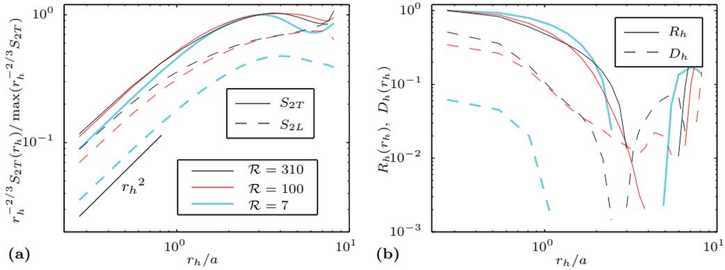
FIG. 6. (a) Compensated transverse and longitudinal horizontal second order structure functions for different  $\mathcal{R}$ . (b) Estimations of the correlations of vertical vorticity  $R_h(r_h)$  and of horizontal divergence  $D_h(r_h)$  normalized by  $\max(R_h(r_h))$ .
