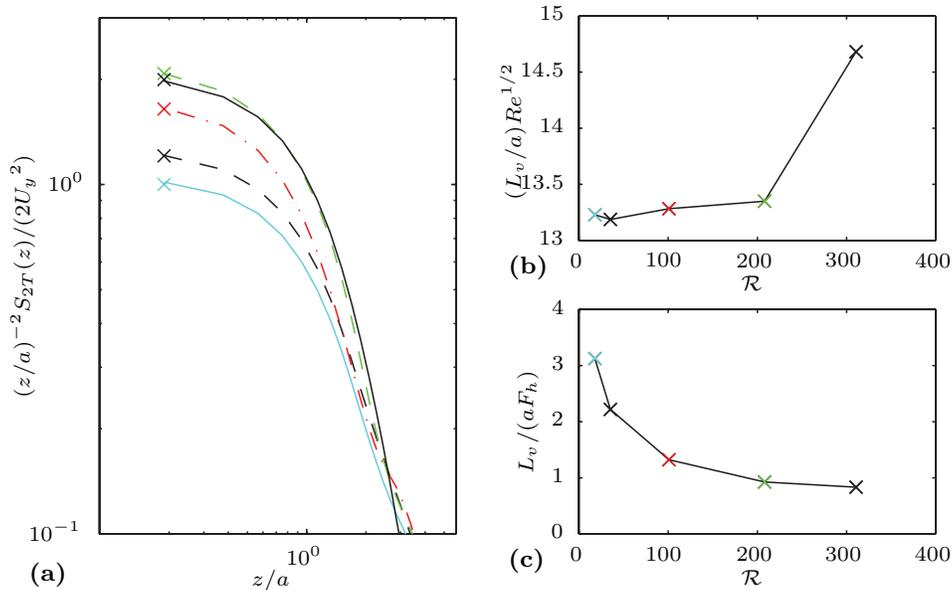
FIG. 5. Variation of the vertical length scale  $L_v$  with  $\mathcal{R}$ . (a) Viscously compensated vertical structure function of order two  $(z/a)^{-2}S_{2T}(z)/(2U_y^2)$  for different  $\mathcal{R}$  (see Figure 4 for the values and representations). The crosses correspond to the values used to compute  $L_v$  for each  $\mathcal{R}$ . (b) rescaled characteristic length scale  $(L_v/a)Re^{1/2}$  and (c)  $L_v/(aF_h)$  as a function of  $\mathcal{R}$ .
