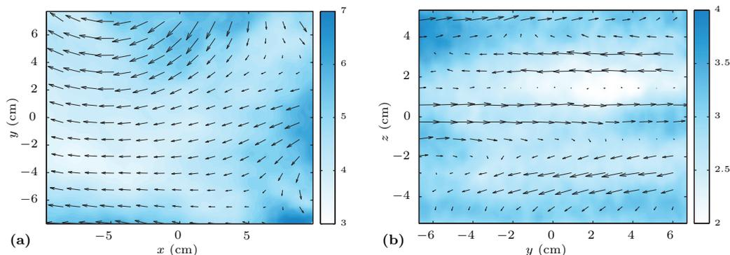
FIG. 8. Horizontal (a) and vertical (b) cross-sections of mean flow  $\mathbf{U}_{//} = \langle \mathbf{u}_{//} \rangle_t$  (arrows) and rms of the velocity fluctuations  $\langle |\mathbf{u}_{//} - \mathbf{U}_{//}|^2 / 2 \rangle_t^{1/2}$  (background shade, in mm/s) for  $\mathcal{R} = 310$ , where  $\mathbf{u}_{//}$  is the velocity parallel to the cross-section. The maximum mean velocity is 12 mm/s in (a) and 4 mm/s in (b).
