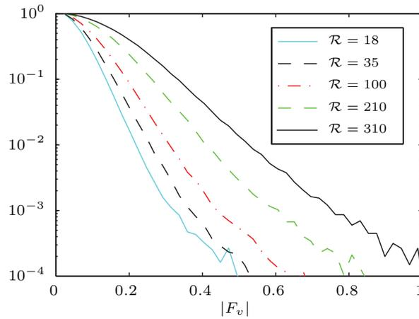
FIG. 4. Normalized probability density function of the local vertical Froude number  $|F_v| = |\omega_x|/(2N) \simeq (4Ri)^{-1/2}$  for various  $\mathcal{R}$  as indicated in the inset. Each curve is normalized by its maximum value.
