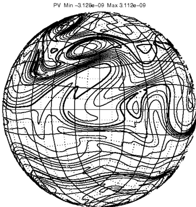
Figure 7. Potential vorticity at day 50 for test case 5 modelled on a cubed-sphere grid of 55296 cells. The contour interval is 2 \times 10^{-10} \text{ s m}^{-2} , and the 0 and \pm 2 \times 10^{-9} contours use double line thickness.
