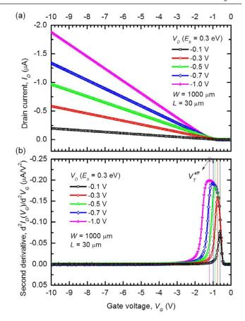
**Figure 2.** (a) Simulated linear-regime transfer characteristics  $I_{\rm D}(V_{\rm G})$  of OFETs with drain voltage  $V_{\rm D}$  as a parameter  $(V_{\rm D}=-0.1,-0.3,-0.5,-0.7$  and -1.0 V). (b) Second derivatives of the simulated  $I_{\rm D}(V_{\rm G})$  which show the effective threshold voltage  $V_{\rm T}^{\rm eff}$  at each peak.
