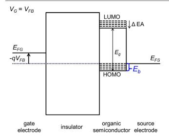
**Figure 3.** Energy diagram based on the metal-insulator-insulator-metal (MIIM) model for various hole injection barrier height  $E_b$ :  $E_b = 0.0, 0.1, 0.2, 0.3, \text{ and } 0.4 \text{ eV}.$
