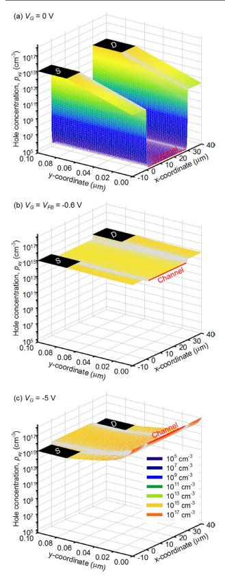
**Figure 5.** Simulated hole concentration in the OFET at different bias conditions: (a)  $V_G = 0$  V, (b)  $V_G = V_{FB} = -0.6$  V and (c)  $V_G = -5$  V. For each condition,  $V_D = 0$  V and  $E_b = 0.3$  eV. The y-coordinate represents the distance from insulator/organic semiconductor interface, while the x-axis is parallel to the interface. The center of channel and the center of source electrode corresponds to x = 15 and x = -5  $\mu$ m.
