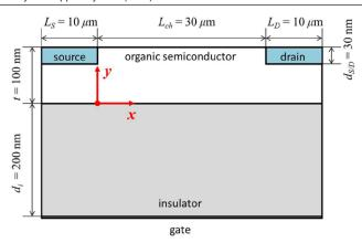
**Figure 1.** Device structure of the OFET which is used in the study, having a BG/TC configuration with geometrical parameters designated in the diagram. Red arrows represent conventional reference axes.
