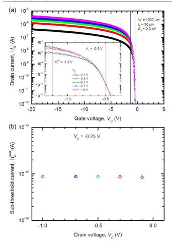
**Figure 7.** (a) Simulated linear-regime transfer characteristics  $I_{\rm D}(V_{\rm G})$  of OFETs in log-scale with drain voltage  $V_{\rm D}$  as a parameter  $(V_{\rm D}=-0.1,-0.3,-0.5,-0.7$  and -1.0 V). (Inset) Close-up of  $I_{\rm D}(V_{\rm G})$  with  $V_{\rm T}=-0.5$  V and  $V_{\rm T}^{\rm eff}=-1.2$  V as a guide to an eye. (b) Sub-threshold current read from  $V_{\rm G}=-0.25$  V for various drain voltage  $V_{\rm D}$ . Hole injection barrier height  $E_{\rm b}$  is 0.3 eV.
