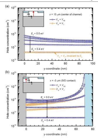
**Figure 6.** Simulated hole concentration across the channel (along y-axis) sectioned (a) at the center of channel ( $x = 15 \mu m$ ) and (b) at the center of source electrode ( $x = -5 \mu m$ ) for two bias conditions:  $V_G = V_{FB} = -0.6 \text{ V}$  and  $V_G = V_T$ . The hole injection barrier height  $E_b$  is varied from 0.0 to 0.4 eV. Accordingly, the value of threshold voltage  $V_T$  varies following the electronic structure of each OFET (figure 4(b)).
