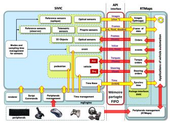
Fig. 5. SiVIC/Types of data managed between SiVIC and RTMaps
