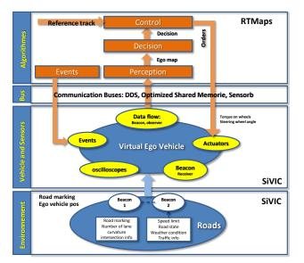
Fig. 7. General diagram of software in the loop model-free controller with functional layers
