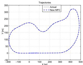
Fig. 1. Reference trajectory versus the closed-loop simulated trajectory
